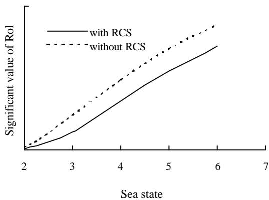
Fig. 9 Roll in beam sea (ship speed 35 kt)
