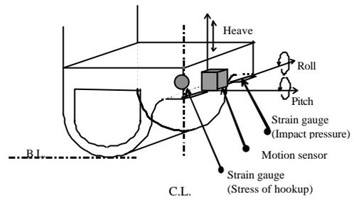
Fig. 3 Arrangement of motion sensor and strain gauge
