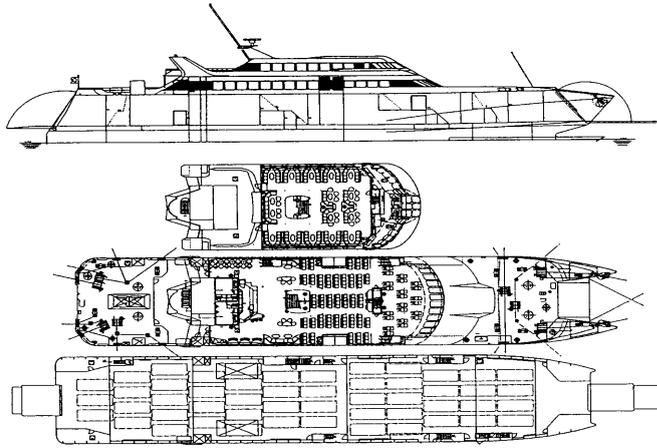
Fig. 1 General arrangement of SSTH-70
