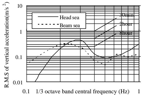
Fig. 10 Motion sickness indices
