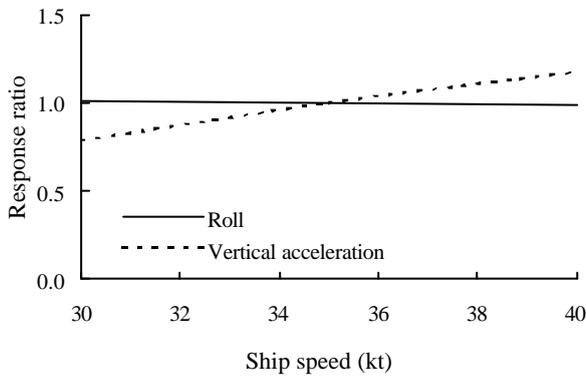
Fig. 7 Roll & vertical acceleration
