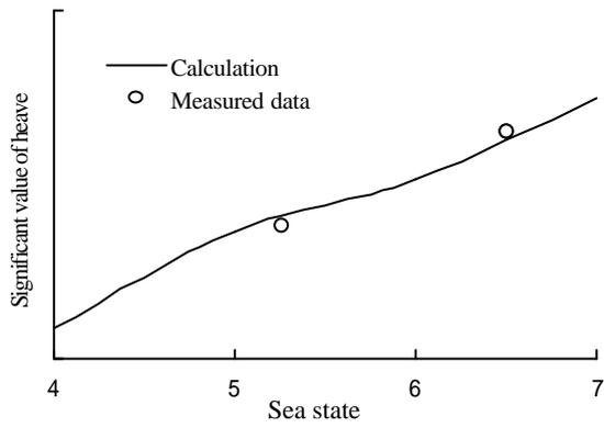
Fig.5 Measured data and calculation results in bow sea
