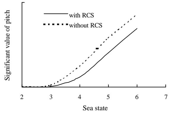
Fig. 8 Pitch in bow sea (ship speed 35 kt)
