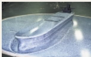
油膜法を用いた船体周囲空気の流動観測 Measuring the flow of air around a hull by the oil film method
