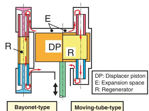
Fig. 3 Comparison of heat exchangers
