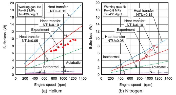
Fig. 13 Buffer loss as a function of engine speed
