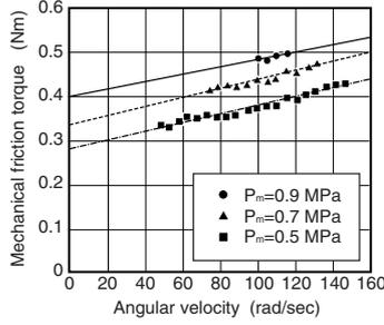
Fig. 12 Friction torque as a function of engine speed
