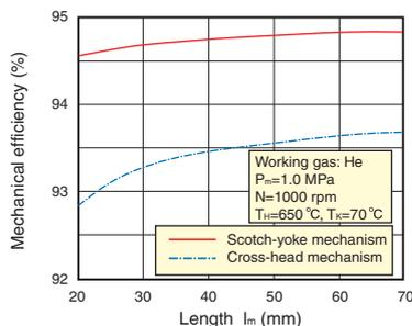
Fig. 6 Mechanical efficiency
