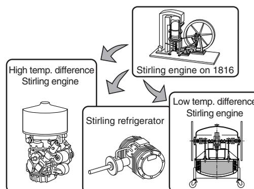
Fig. 1 Stirling cycle machines
