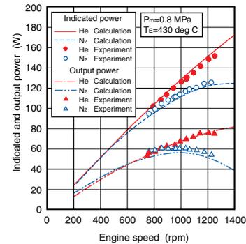
Fig. 15 Power as a function of engine speed
