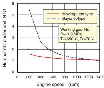
Fig. 4 Number of transfer units function as engine speed
