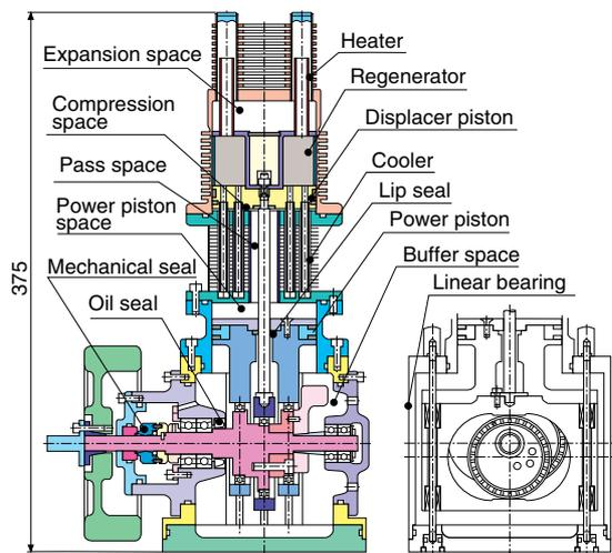
Fig. 7 Schematic view of the prototype engine
