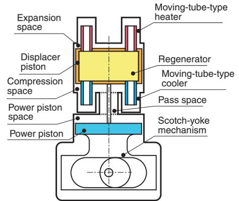
Fig. 2 Basic structure of the prototype engine
