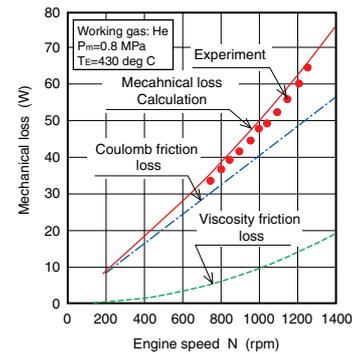
Fig. 14 Mechanical loss as a function of engine speed
