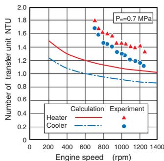
Fig. 10 Number of transfer units as a function of engine speed
