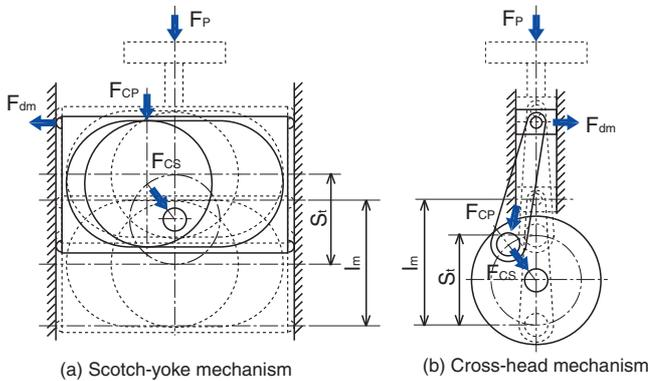
Fig. 5 Comparison of piston drive mechanisms
