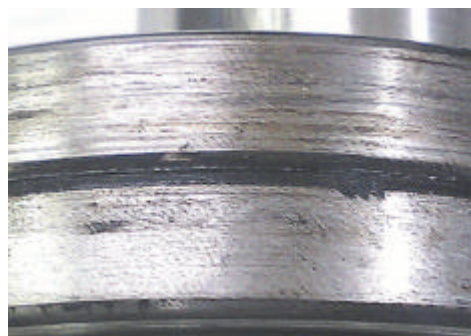
Figure 5, Outer Ring Surface of Ball Bearings for Wear or Scarring after 500 hr Operating.
