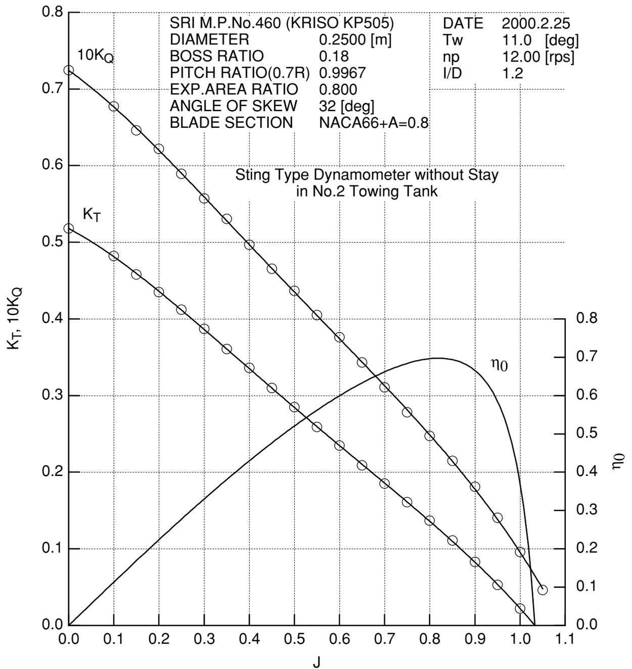
**Fig. 3 Propeller Open Characteristics of Tested Propeller Model**
