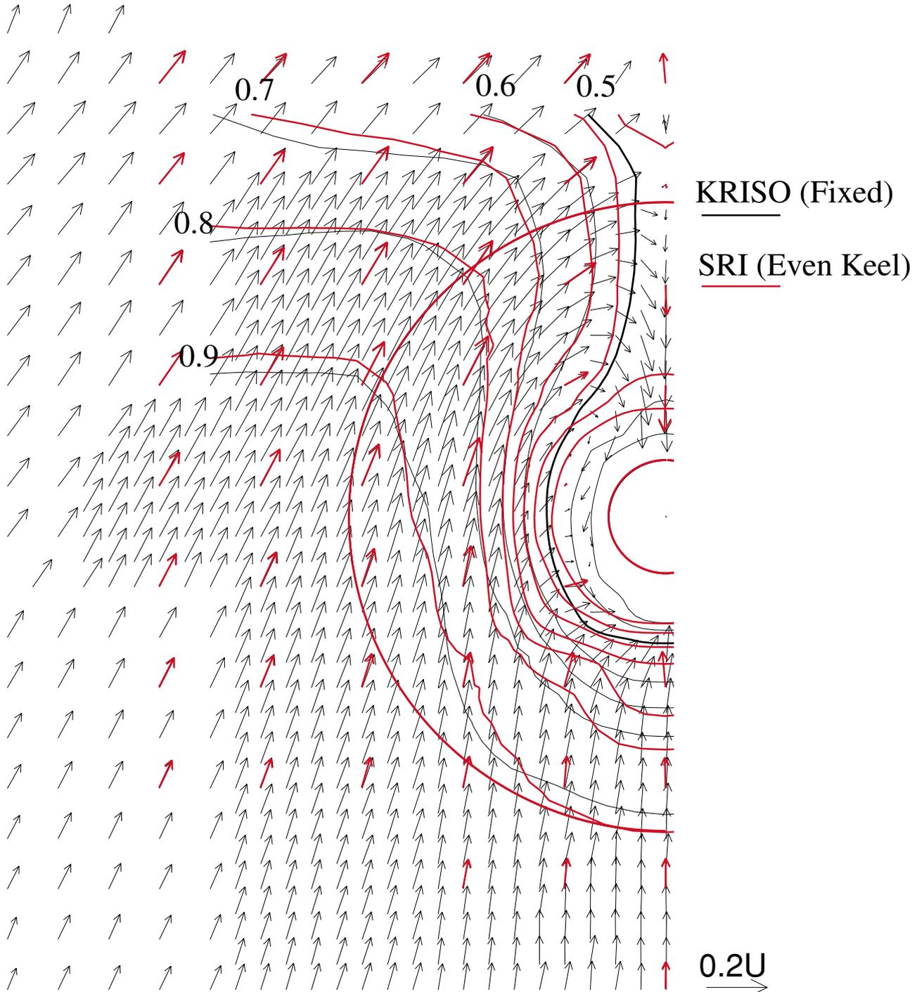
**Fig. 6 Comparison of Local Velocity Field Measurements in the Propeller Plane
