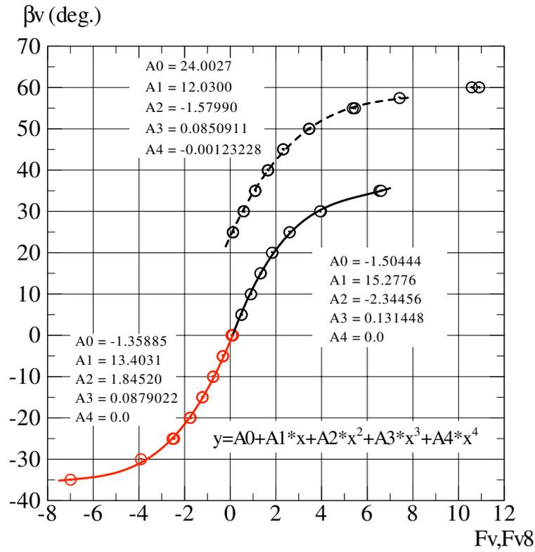
(c) Correlation Curves of Vertical Flow Angle  $\beta_v$  versus F<sub>v</sub> and F<sub>v8</sub>
