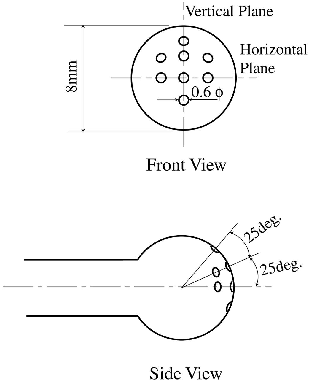
**Fig. 4 Geometrical Shape of Eight-Hole Pitot Tube**
