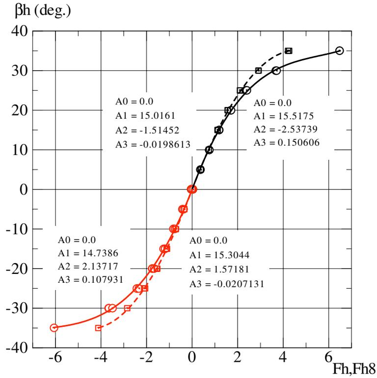
(a) Correlation Curves of Horizontal Flow Angle  $\beta_h$  versus  $F_h$  and  $F_{h8}$
