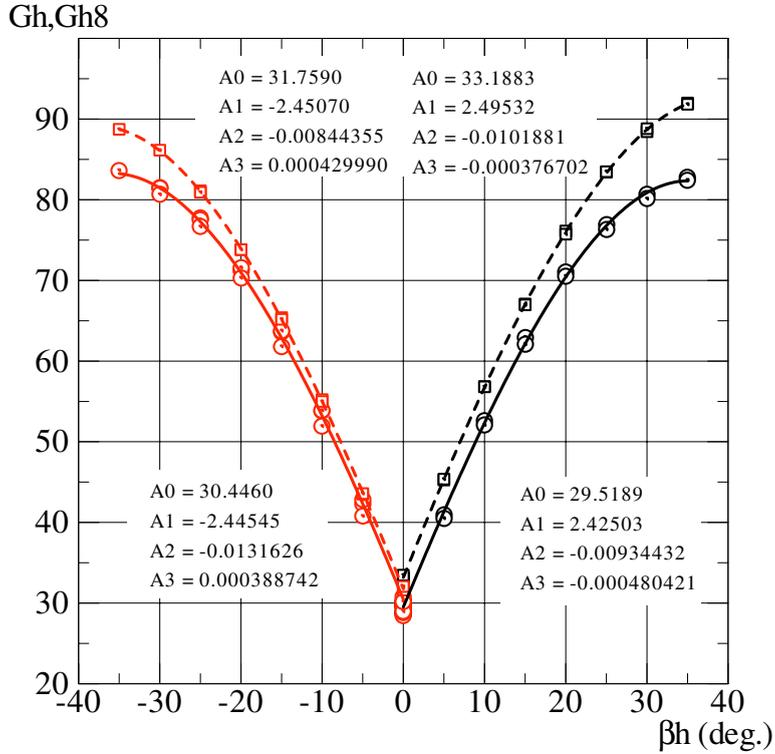
(b) Correlation Curves of  $G_h$  and  $G_{h8}$  versus Horizontal Flow Angle  $\beta_h$
