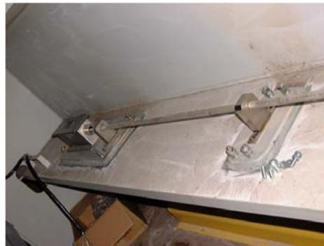
b) Long-base strain meter below upper deck
