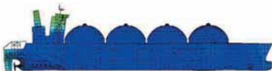
振動解析用全船FEM model
