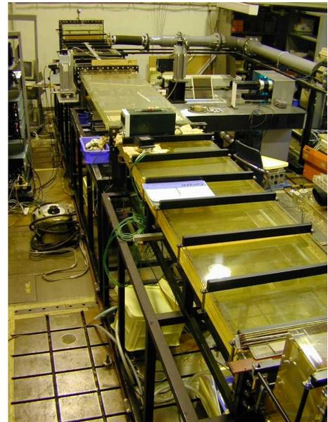
Fig. 2a. Schematic diagram of two dimensional water channel Inner height:  $H=40\text{mm}$ , width:  $W=500\text{mm}$ . All the measurements were made at  $x=3000\text{mm}$ .
