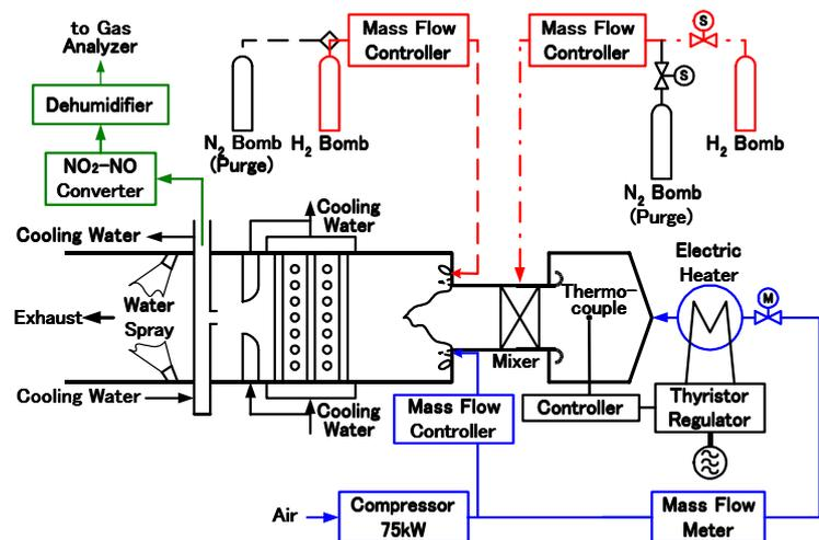
Fig. 1 Schematic Flow Sheet of Test System
