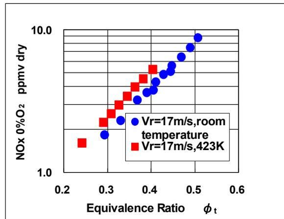
Fig. 7 Effects of Inlet Air Temperature of the Combustion Air on NOx Emissions
