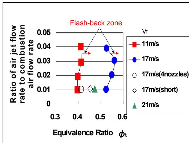
Fig. 3 Deterrent Effect of Air Jet to Flash-back
