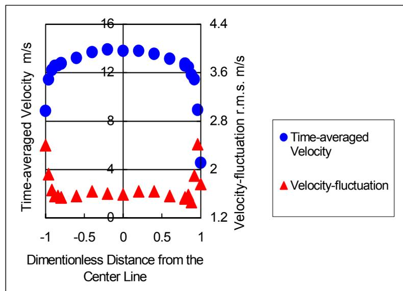
Fig. 4 Distributions of Mean Velocity and Fluctuation
