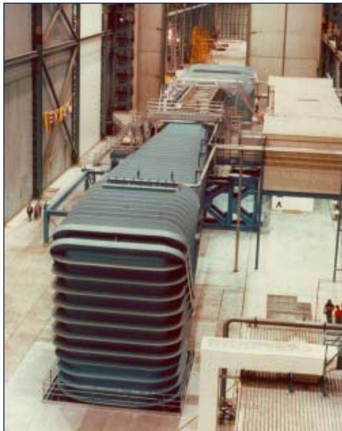
Figure 1a. The US Navy's Large Cavitation Channel. The LCC is the world's largest water flow facility. Note the size of the people at the left and right edges of this picture.
