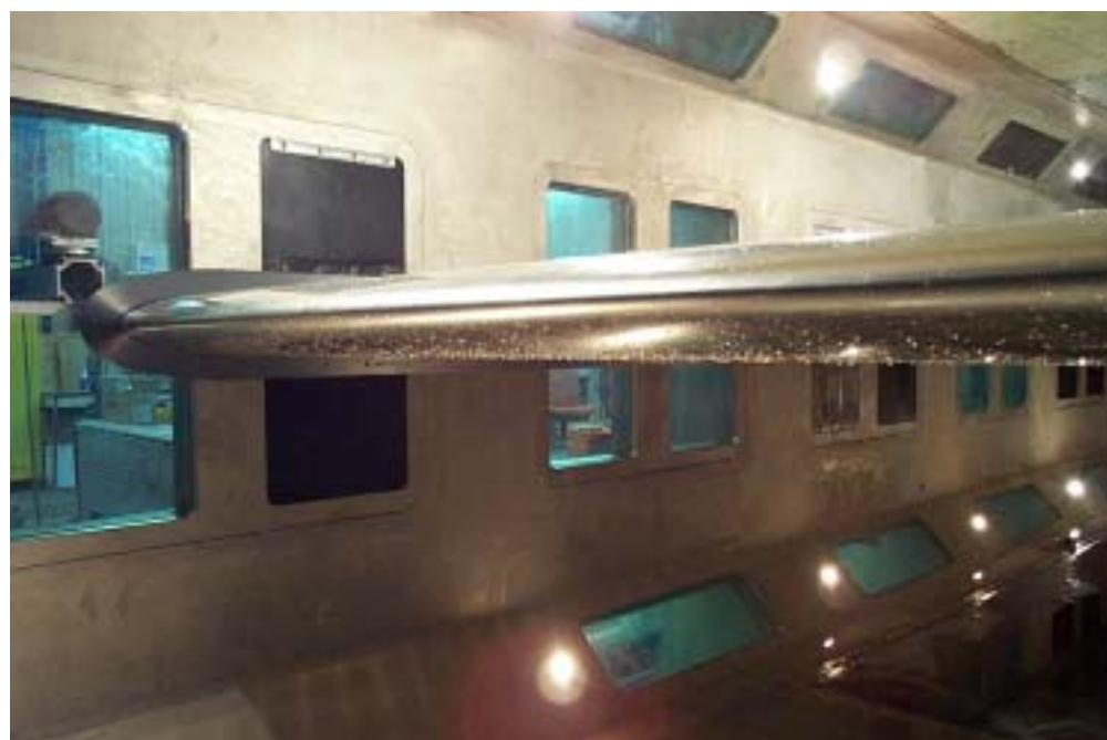
Figure 6b: Polished nose section (4:1 ellipse) of the HIPLATE model as seen mounted in the LCC.
