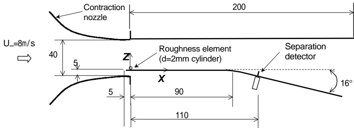
Fig.1 Schematic of wind tunnel and test section with a separation detector and roughness element installed on the test plate.
