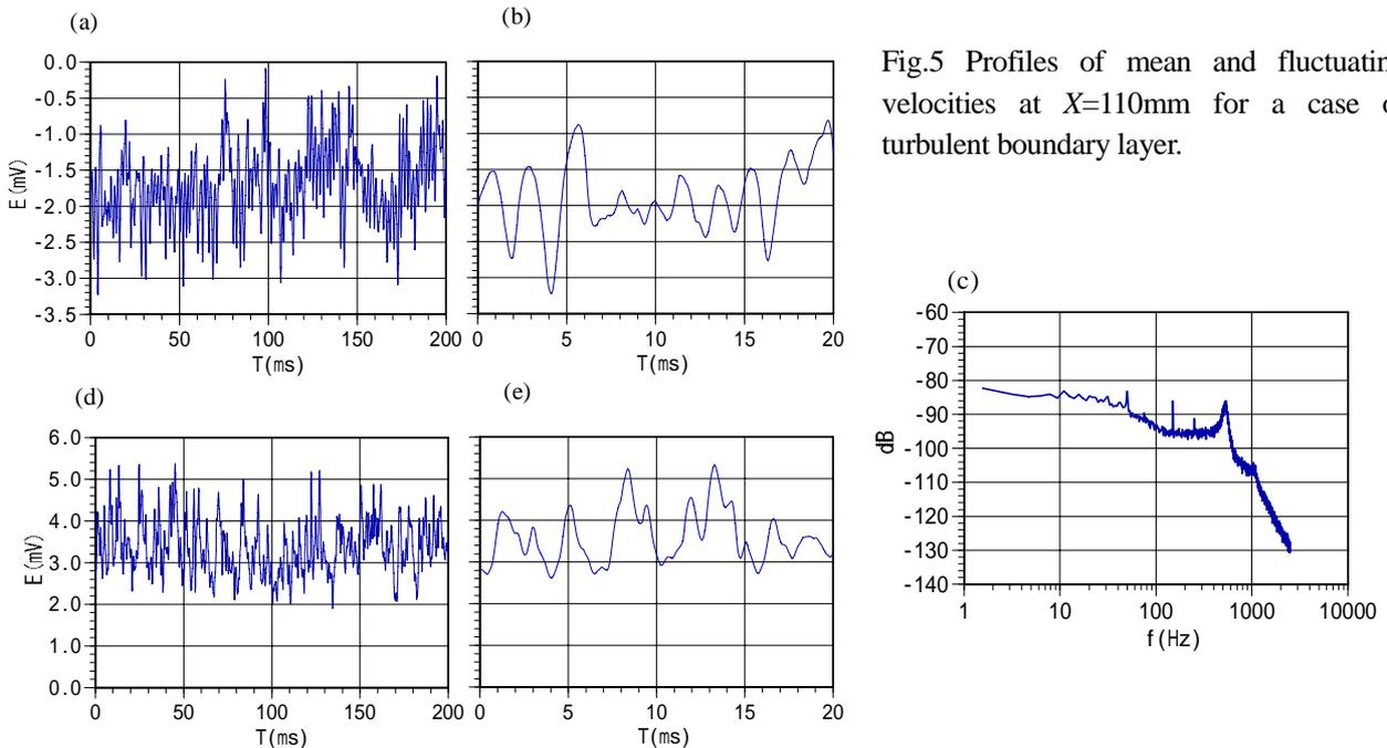
Fig.6 Separation detector signal and power spectrum at  $X=110\text{mm}$ .
