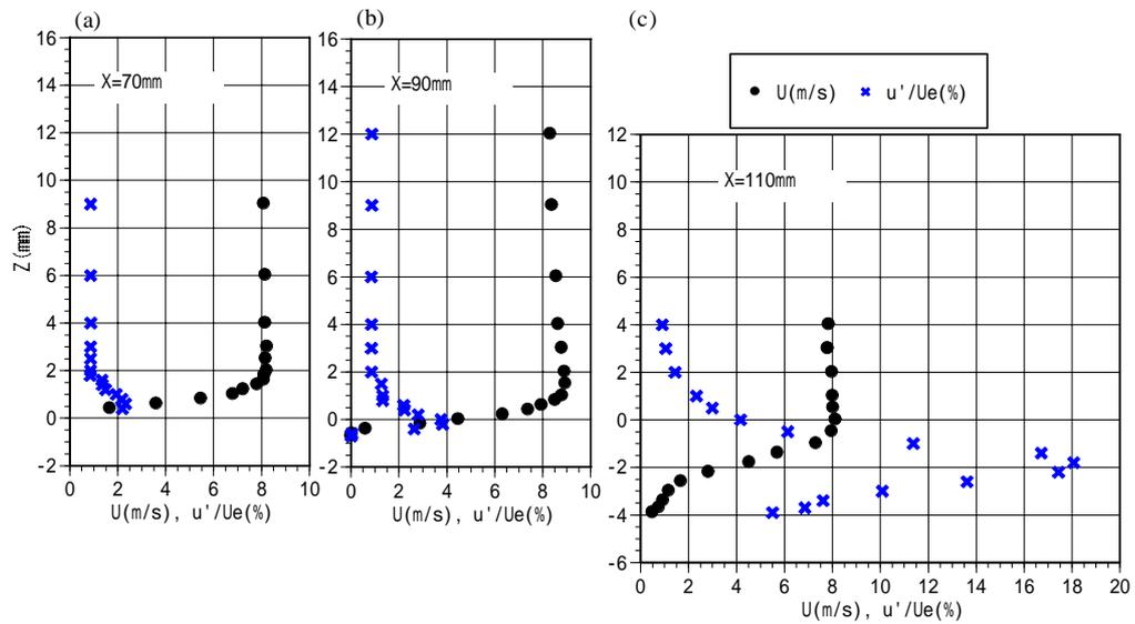
Fig.2 Profiles of mean and fluctuating velocities at three locations for a case of laminar boundary layer at the leading edge.
