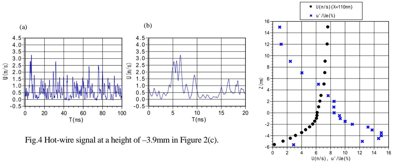
Fig.4 Hot-wire signal at a height of  $-3.9\text{mm}$  in Figure 2(c).
