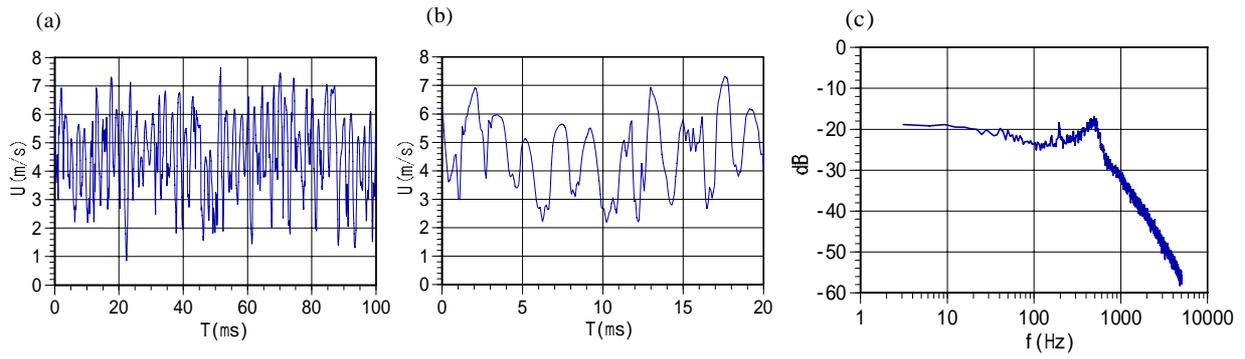
Fig.3 Hot-wire signal captured at the peak of velocity fluctuation at  $X=110\text{mm}$ .
