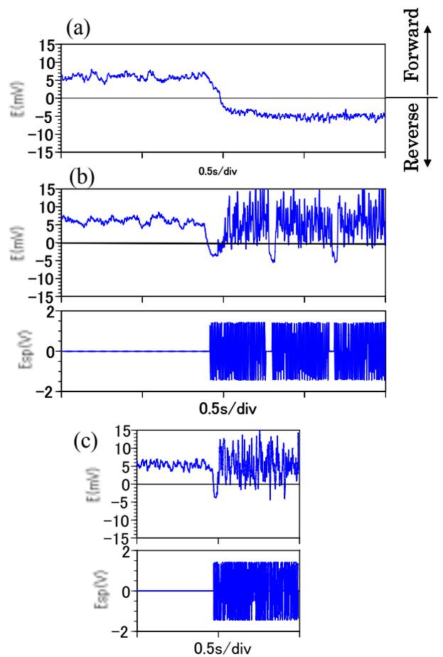
Fig.10 Demonstration of the control system for the stepwise changed flow field. (a) Without excitation, (b) With excitation, the acquisition time is 32ms, (c) With excitation, the acquisition time is 3.2ms,
