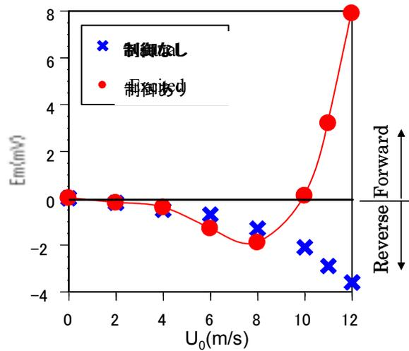
Fig.8 Time-averaged CS output for various free-stream velocity.
