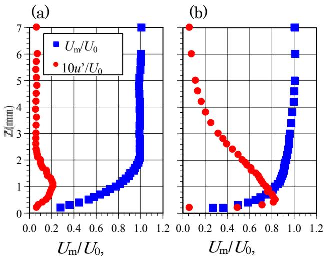
Fig.5 Profiles of mean velocity,  $U_m$ , and turbulence intensity,  $u'/U_0$ , at  $x=170\text{mm}$  and  $U_0=10\text{m/s}$ . (a) Natural, (b) Excited
