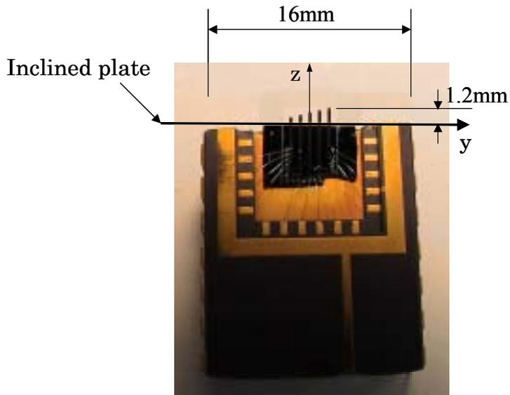
Fig.2 Cantilever sensor (Ozaki et al. 2000).
