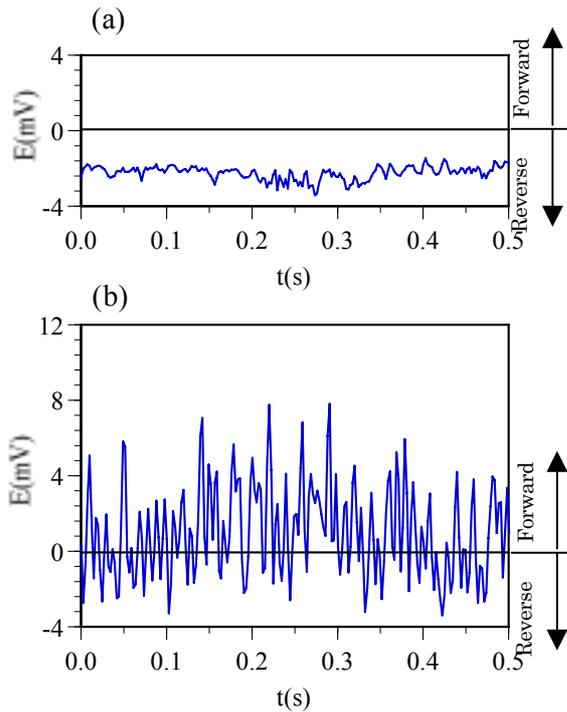
Fig.7 Instantaneous waveforms of Cantilever sensor output at  $U_0 = 10\text{m/s}$ . (a)Natural , (b)Excited
