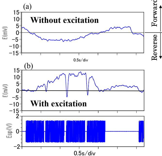
Fig.9 Demonstration of the control system. (a) CS output without excitation, (b) CS output and speaker driving pulse,  $E_{sp}$ , with excitation.
