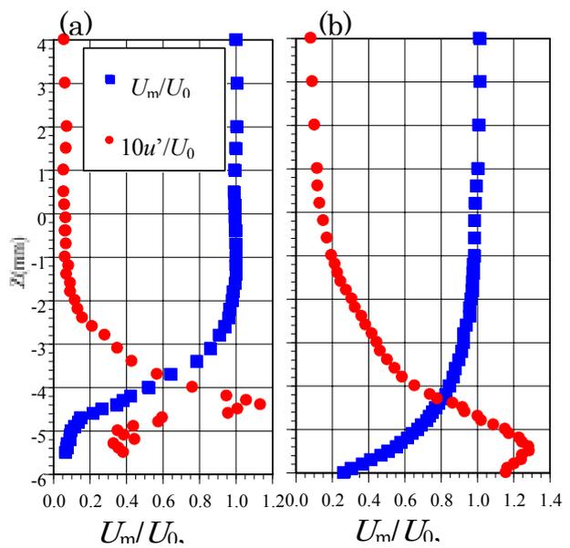
Fig.6 Profiles of mean velocity,  $U_m$ , and turbulence intensity,  $u'/U_0$ , at  $x=215\text{mm}$  and  $U_0=10\text{m/s}$ . (a) Natural, (b) Excited
