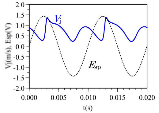
Fig.3 Time traces of the speaker driving pulse,  $E_{sp}$ , and hot-wire output,  $V_j$ , measured above the hole ( $z=1\text{mm}$ ) for no wind.
