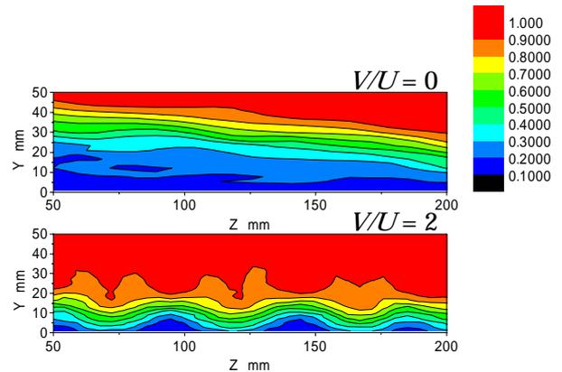
Fig.8 Velocity contour of boundary layer at trailing edge  $\alpha = 4^\circ$
