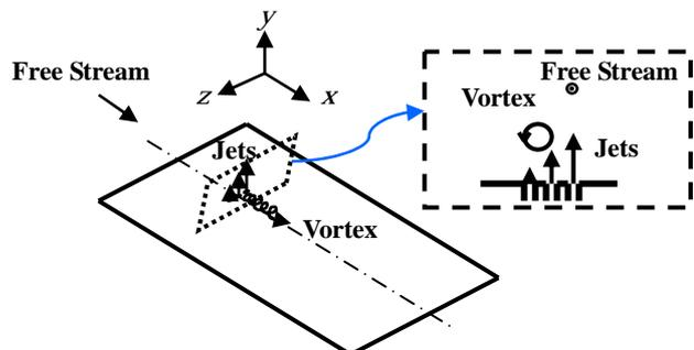
Fig.1 Principle of jet type VG.
