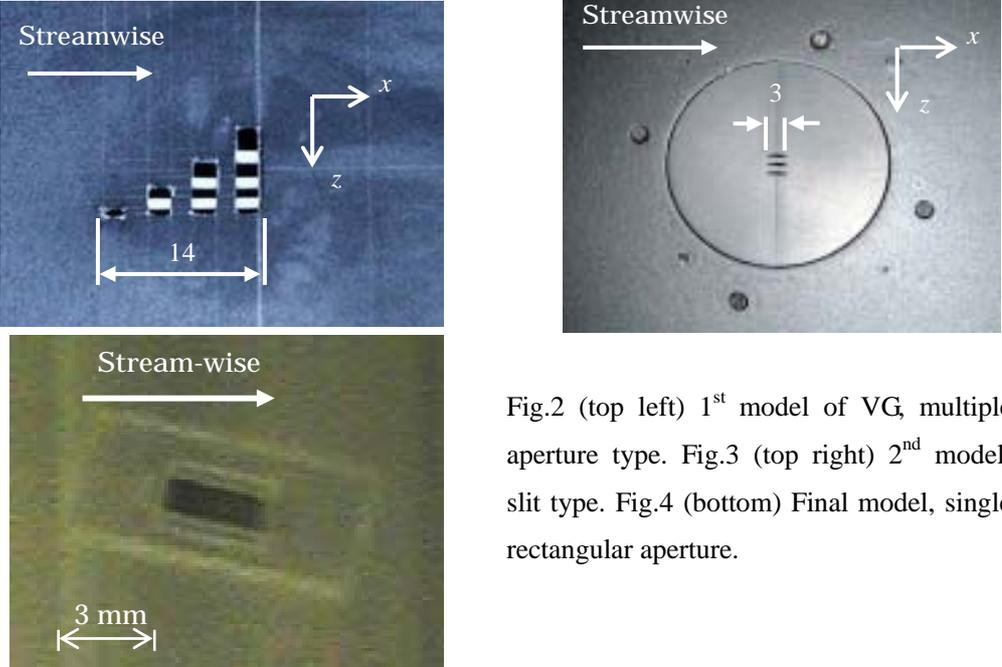
Fig.2 (top left) 1<sup>st</sup> model of VG, multiple aperture type. Fig.3 (top right) 2<sup>nd</sup> model, slit type. Fig.4 (bottom) Final model, single rectangular aperture.
