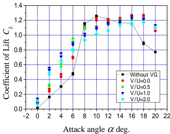
Fig.7 Effect of the VG at leading edge on  $C_L$
