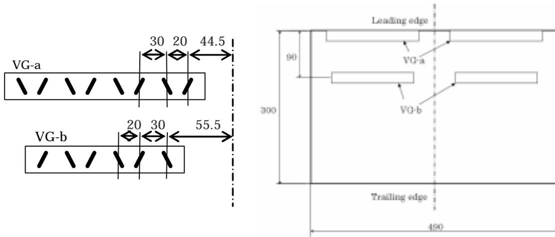
Fig. 6 Arrangement of the vortex generator on the wing
