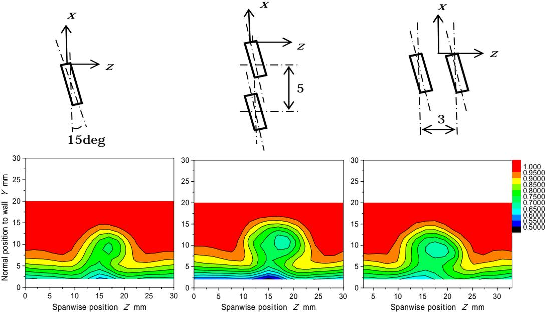
Fig.5 (a) (left) Contour of boundary layer velocity by 1 aperture. (b) (middle) 2 apertures set stream-wise with 5 mm pitch. (c) (right) 2 apertures set spanwise with 3 mm pitch.
