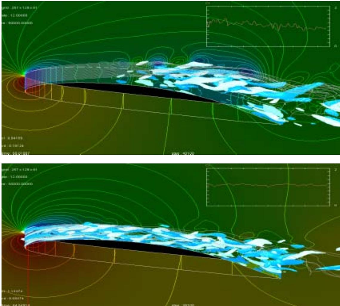
Fig. 9 Flow field around MEL001 airfoil.  $Re=50,000$ ,  $\alpha=6^\circ$ . (a) (top) without VG (b) (bottom) with VG at the leading edge.  $V_{jmax}/U=1$ . Inset: lift coefficient as a function of time, full scale is about 1 sec (Yoshida, et al. 2005).
