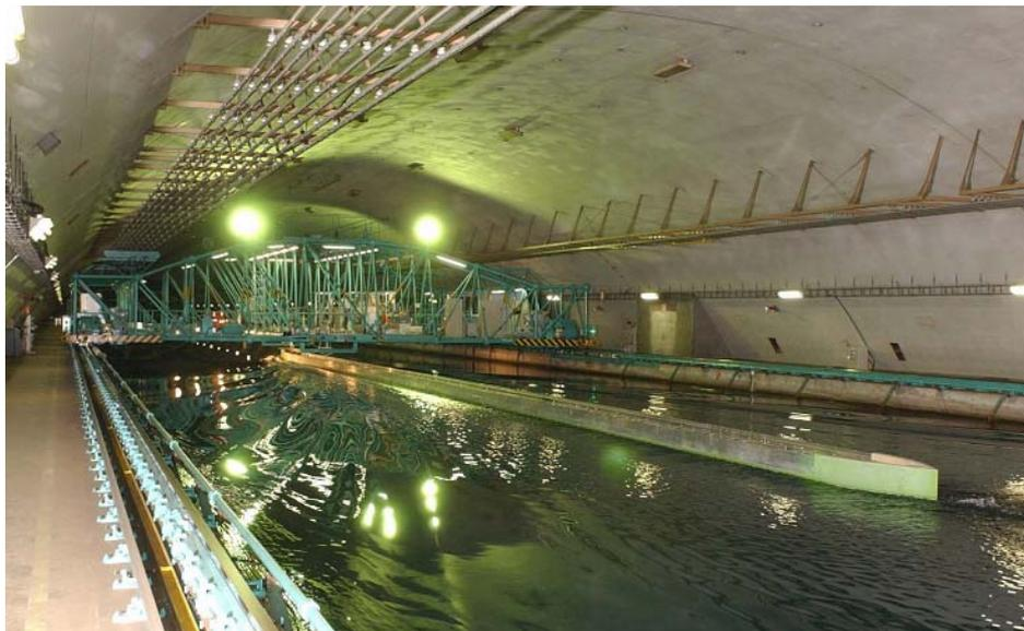
Fig. 6 A 50 m-long flat plate towed in a 400 m-long towing tank for microbubble experiment.
