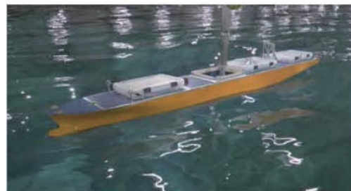
Hazardous Event Reproduction Test in Short Crested Irregular Waves (Research on Fluid Dynamic Performance Evaluation for Safe Navigation of Ships)
