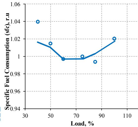
Steady-state performance of the prototype engine is mapped fairly-well.
