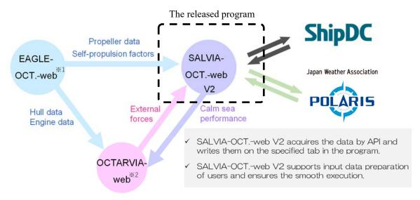
\*1 EAGLE-OCT.-web: Calculation program to estimate the hull form and the calm sea performance from the principal dimensions which is used for the input data of the above programs
