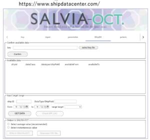
Request view in SALVIA-OCT.-web V2 for the acquisition of onboard monitoring data stored in ShipDC
