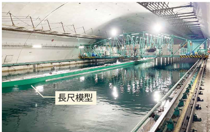
36m-long model experiment (400m tank)
