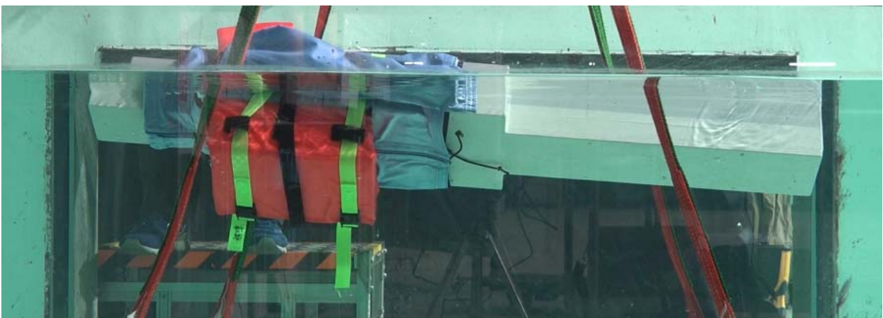
Experiment using dummy with clothing and reduced-size lifejacket (during turning)
