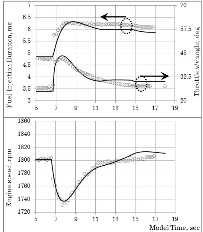
Fig.3 Transient response during step load input.
