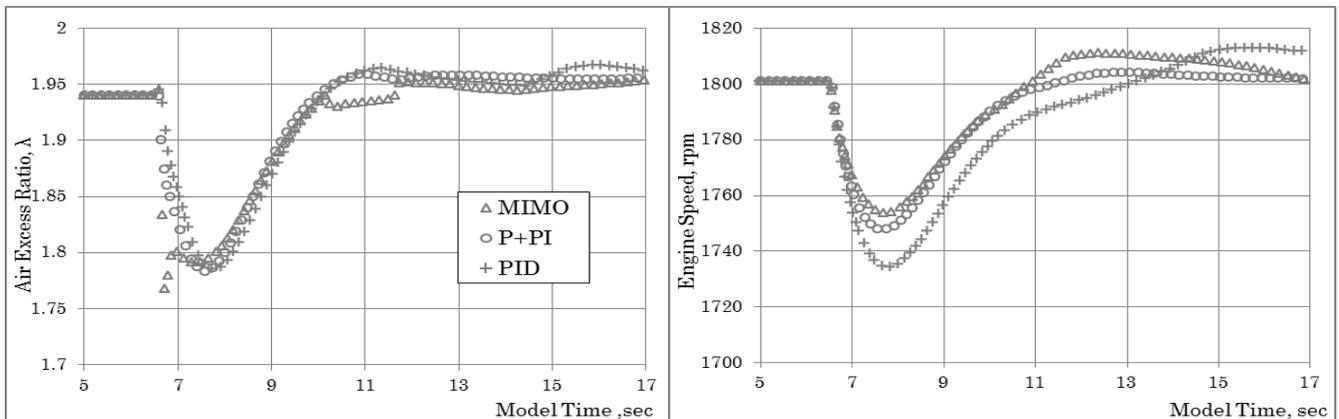
Fig.4 Effect of different control strategies on the gas engine transient dynamic
