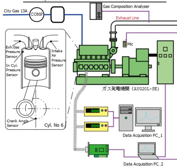
Fig.1 Engine data acquisition system
