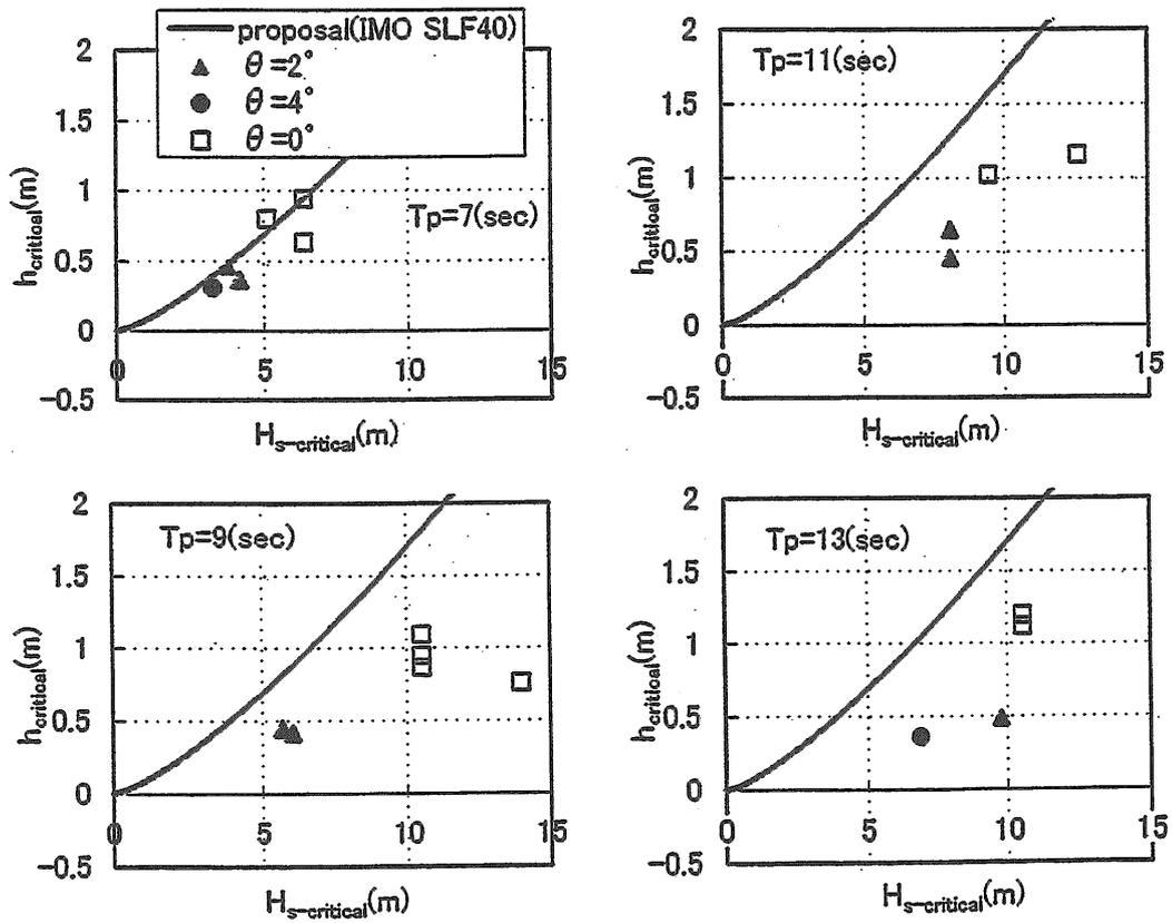
Fig.3.11 Effect of Peak Period of Wave Spectrum to Critical Significant Wave Height (Designed Deck Height)
