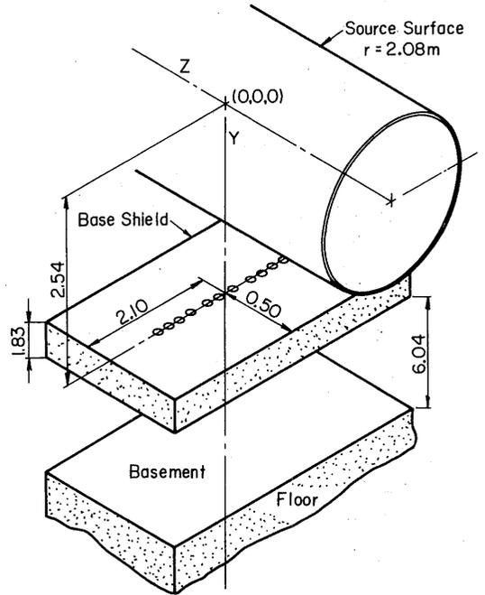
Fig. 21 Schematic representation of the three-dimensional mode for the Monte Carlo diagnostic basement penetration calculation.<sup>62)</sup>
