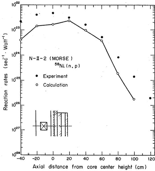
Fig. 9 Comparison of MORSE reaction rates of  $^{58}\text{Ni}$  (n,p) with measured values along the dotted line given in Fig. 6 of N-II-2<sup>33)</sup>
