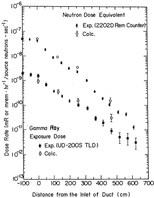
Fig. 12 Distribution of the total neutron dose equivalent and gamma ray exposure dose along the duct.<sup>36)</sup>
