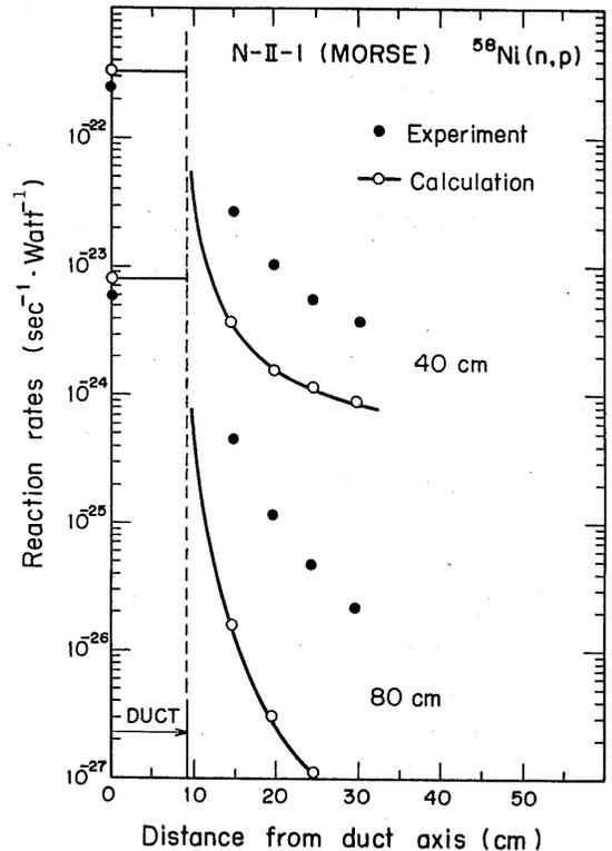
Fig. 8 Comparison of MORSE reaction rates of  $^{58}\text{Ni}$  (n,p) with measured values at radial distances of 41 and 81 cm from duct mouth of N-II-1<sup>33)</sup>
