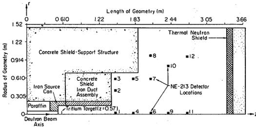
Fig. 19 Two-dimensional calculational model of the experimental configuration.<sup>59)</sup>
