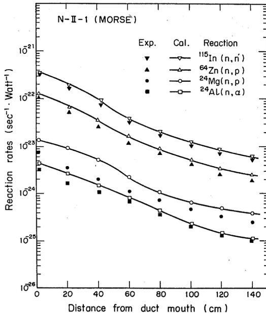
Fig. 7 Comparison of MORSE reaction rates with measured values along duct axis of N-II-1<sup>33)</sup>
