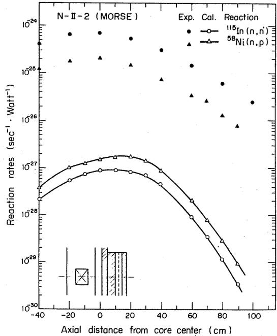
Fig. 10 Comparison of MORSE reaction rates with measured values along the dotted line in Fig. 6 of N-II-2<sup>33)</sup>
