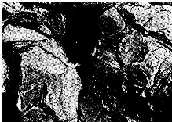
Photo 4 Replication electron fractographs of HAZ root cracks developed in cruciform-shaped specimens.
