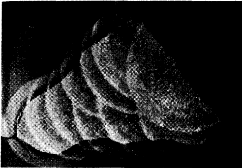
Photo 1 Various welding cracks developed in cruciform-shaped specimen of steel B30 (x2)
