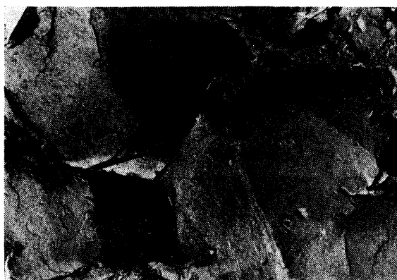
Photo 3 HAZ root crack developed in eight pass welded tee-shaped specimen of steel NA20.
