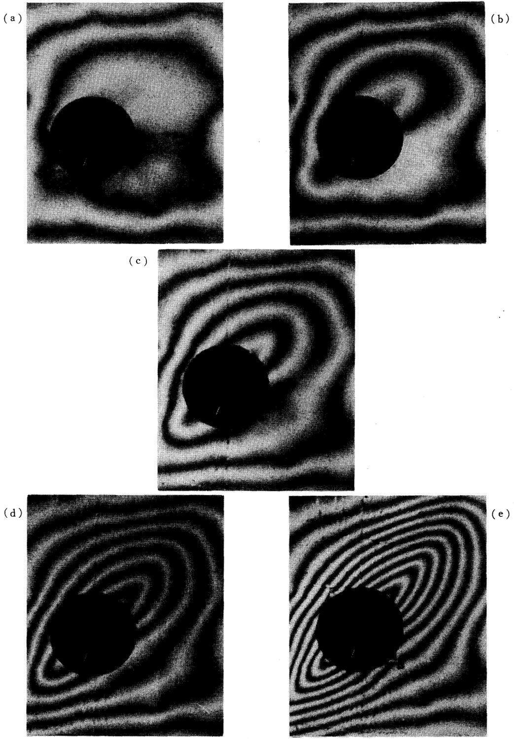
**Photo 3** Contour line system of the deflection surface (SI 350=3.2-90φ)
