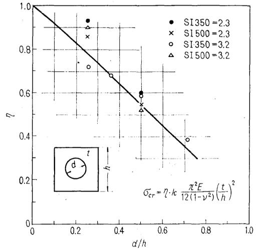
Fig. 14 Critical shearing stress versus opening ratio
