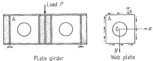
Fig. 1 Test layout of plate girder
