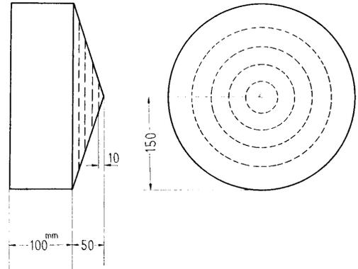
Fig. 6 Cone model for calibrating moiré pattern
