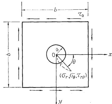
Fig. 2 Square plate with central circular hole
