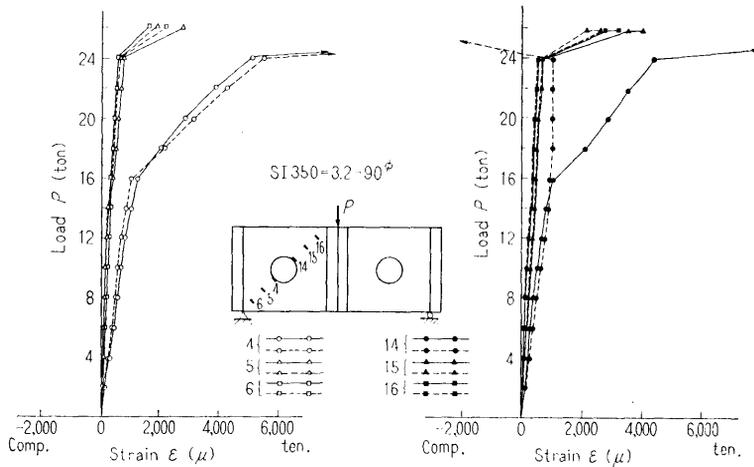
Fig. 10 (b) Load-strain curves
