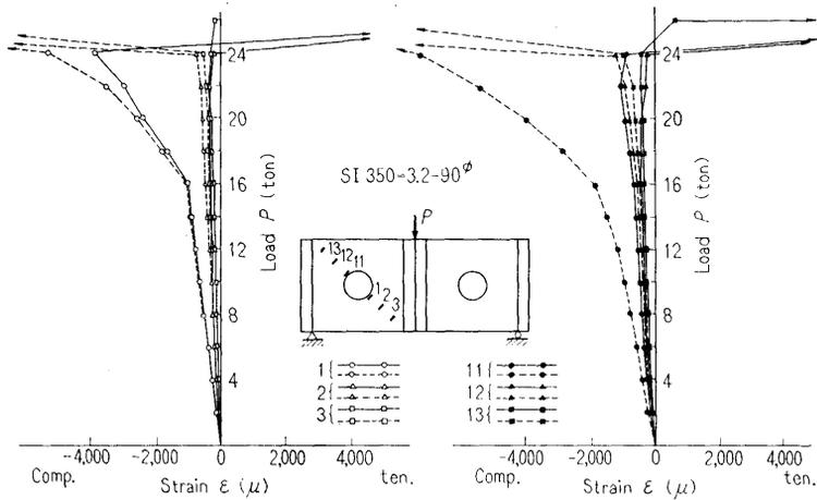
Fig. 10 (a) Load-strain curves
