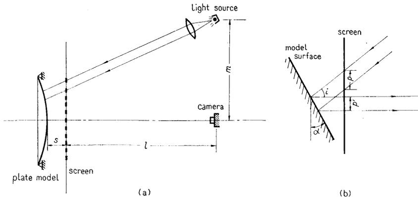
**Fig. 5** Schematic representation of moiré method
