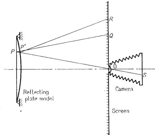
**Fig. 4** Principle of Ligtenberg's method
