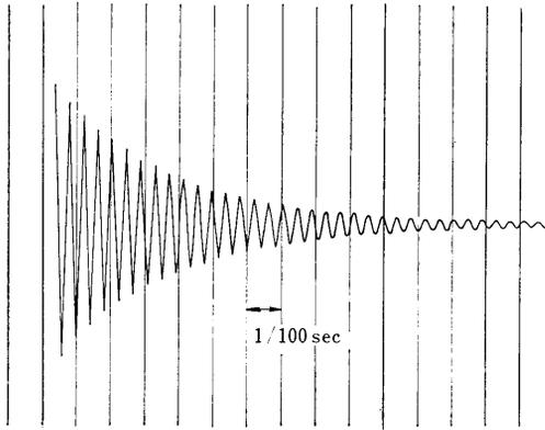
Fig. 13 Record of Free Vibration of Water Pressure Gage
