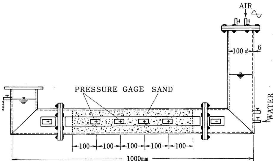
Fig. 10 Details of Dynamic Permeameter
