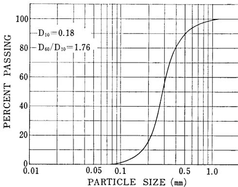
Fig. 15 Grain-Size-Accumulation Curve of Specimen I
