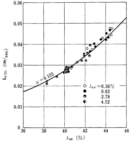
Fig. 2 Relationship between Permeability and Effective Porosity
