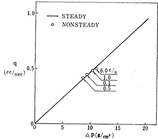
Fig. 18 Comparison between Quantity of Seepage in Steady State and Non-steady State
