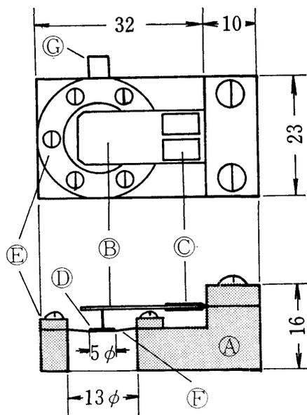
Fig. 12 Details of Water Pressure Gage
