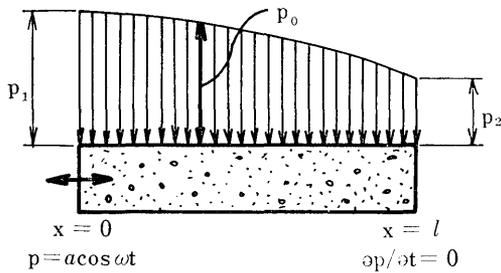
Fig. 6 Boundary Conditions and Diagram of Static Pressure Distribution in Steady State
