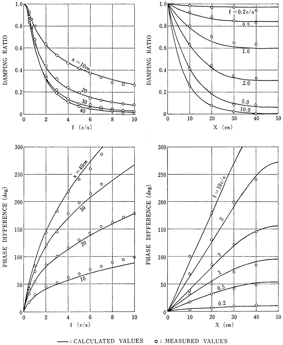
Fig. 19 An Example of Damping Ratio and Phase Difference of Seepage Pressure for  $f$  and  $x$  (Specimen I,  $\lambda=44\%$ ,  $\bar{\lambda}_{a0}=2.78\%$ ,  $\bar{\lambda}'_{a0}=6.32\%$ ,  $l=50$ cm,  $\partial p/\partial t=0$  at  $x=l$ )
