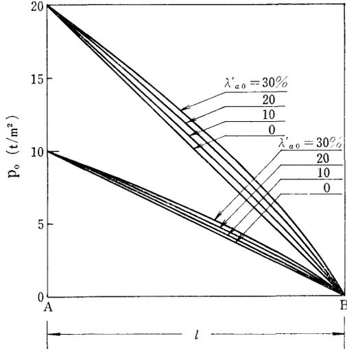
Fig. 3 Distribution of Seepage Pressure in Porous Media Contained Air Bubbles in Steady State ( $\lambda=40\%$ )
