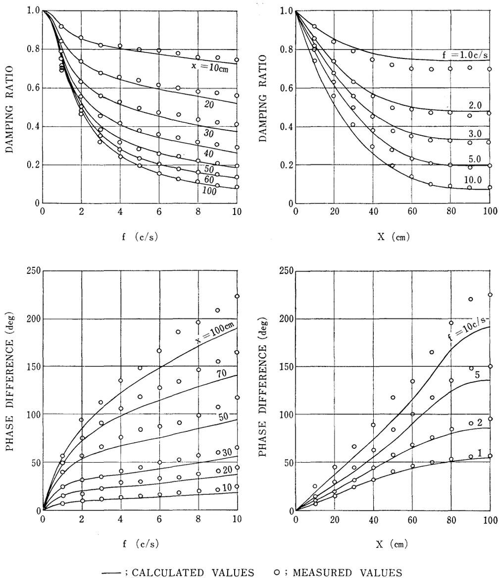
Fig. 20 An Example of Damping Ratio and Phase Difference of Seepage Pressure for  $f$  and  $x$  (Specimen II,  $\lambda=37.6\%$ ,  $\bar{\lambda}_{a0}=1.21\%$ ,  $\bar{\lambda}'_{a0}=3.20\%$ ,  $l=100\text{cm}$ ,  $\partial p/\partial x=0$  at  $x=l$ )
