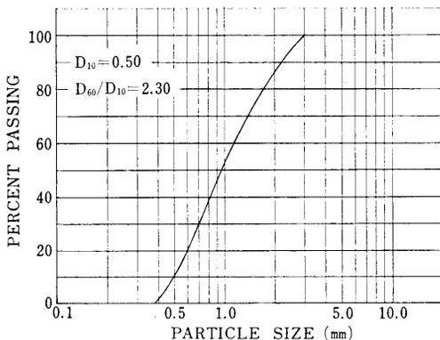
Fig. 16 Grain-Size-Accumulation Curve of Specimen II
