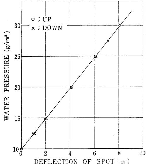
Fig. 14 Calibration of Water Pressure Gage
