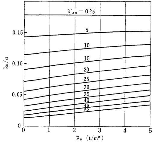
Fig. 4 Relationship between Pressure and Permeability by Eq. (3) ( $\lambda=40\%$ )
