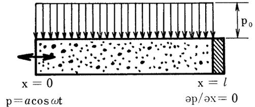
Fig. 5 Boundary Conditions and Diagram of Static Pressure Distribution
