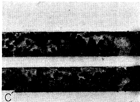
Photo 4 Test Pieces after Corrosion (Effect of Immersion Ratio, \theta=35^\circ\text{C} , f_\sigma=15 CPM, \delta=5 mm) * aa', bb', and cc' show both sides of the same pieces.
