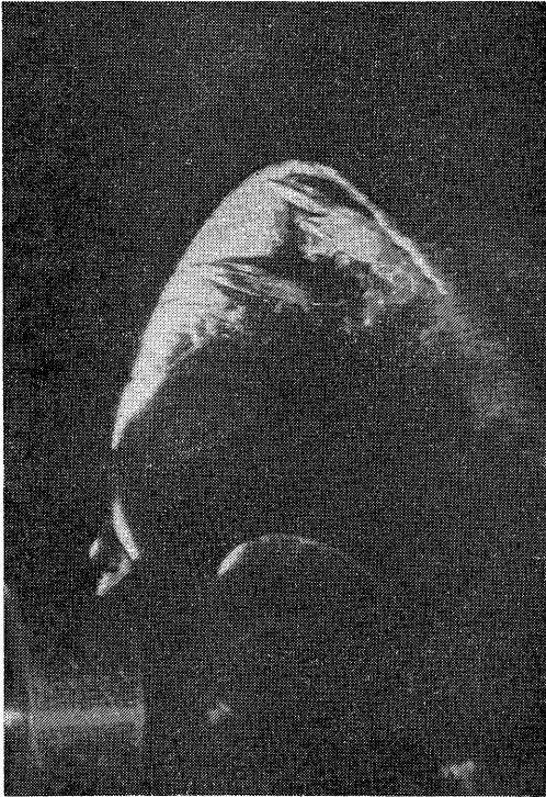
Fig. 30C An Example of Cavitation Pattern Unfavorably Influenced by the Existence of Pin ( \theta=0^\circ )
