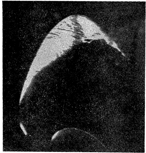
Fig. 14 Photos of Cavitation Pattern on MP-1 Propeller with Roughness at Full Load Condition
