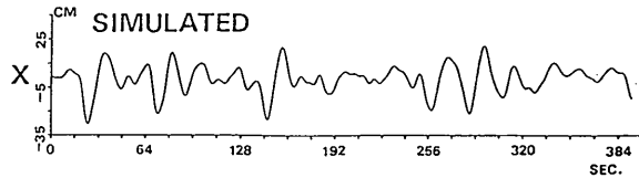
Fig. 14 Comparisons in time domain between simulated low frequency motions and measured results of surge motion
