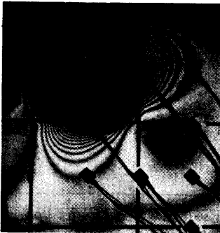
Photo 9 Deformation of outer plate (Model S-III, (ii))
