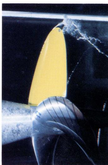
Photo 10 M. P. No. 229 in Cloud Cavitation Condition II ( $\sigma_n = 1.95$ ,  $\Theta = 60^\circ$ )
