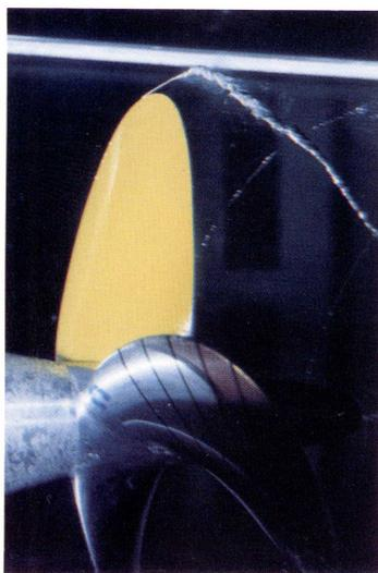
Photo 9 M. P. No. 229 in Cloud Cavitation Condition I ( $\sigma_n = 2.92$ ,  $\Theta = 60^\circ$ )
