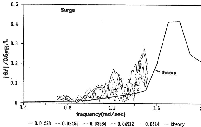
Fig. 4.12 b) Amplitude of QTF of second order slow drift force to mean wave frequency  $\Omega_1$  of two wave components
