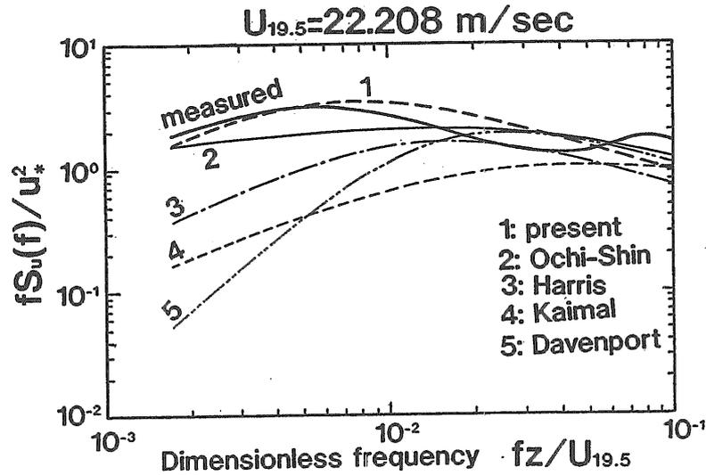
Fig. 3.8 Comparison between measured wind spectrum and other proposed spectrum forms
