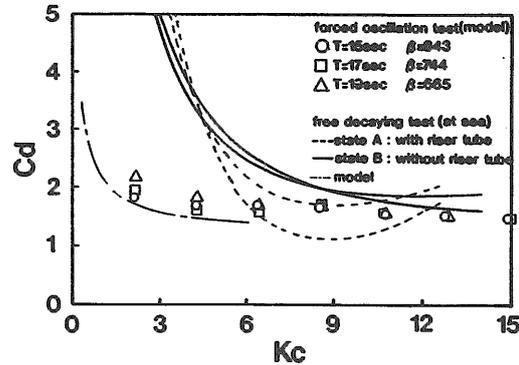
Fig. 4.7 Keulegan-Carpenter number dependence of sway drag coefficient
