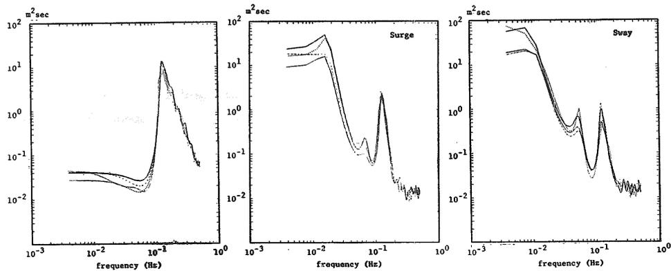
Fig. 3.4 Examples of wave, surge and sway spectra
