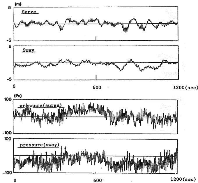
Fig. 3.5 Time histories of surge, sway and wind pressure fluctuations in surge and sway directions
