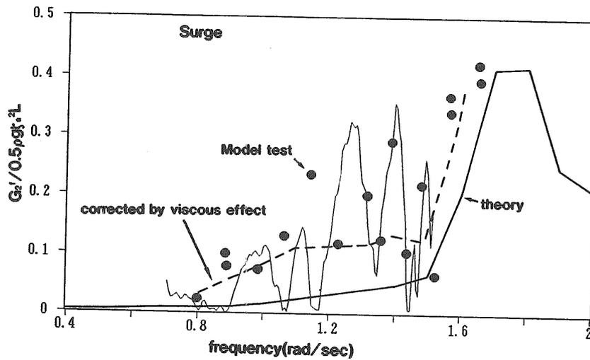
Fig. 4.12 a) Steady drift force coefficient to wave frequency  $\omega (= \Omega_1)$
