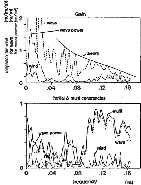
Fig. 3.9 Gains of frequency response function, partial and multiple coherencies among surge motion and wave, instantaneous wave power and wind pressure fluctuation in head sea and wind (The "theory" in the upper figure means the the calculated line based on the first order potential theory and the "multi" in lower figure represents the multi coherency)
