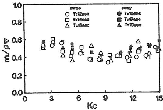
Fig. 4.3 Surge added mass coefficient obtained from forced oscillation test of "POSEIDON" model
