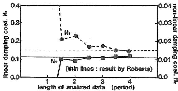
Fig. 4.1 Comparison between the present identification result and the identification one by Roberts[13] with respect to estimation of damping coefficients from ship roll data ( In this case, the damping force model is assumed as;  $N_1\dot{X} + N_2\dot{X}|\dot{X}|$ )
