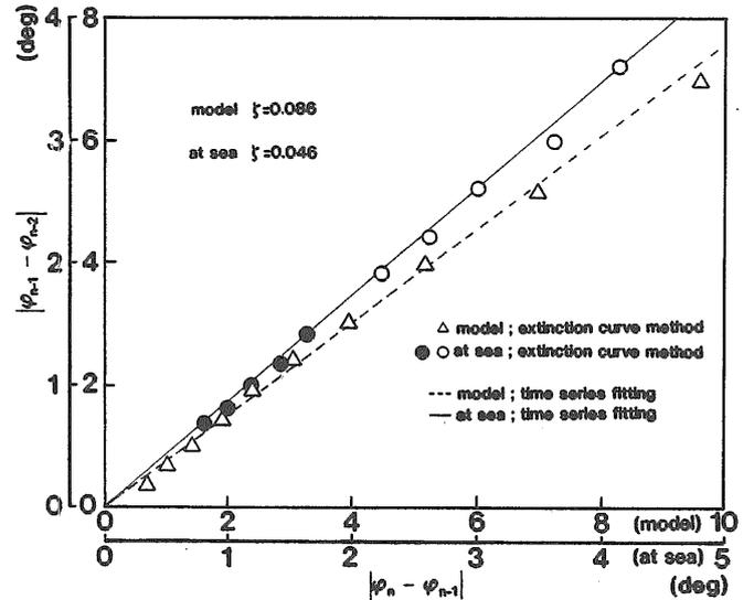
Fig. 4.10 Extinction curve of full-scale roll decaying motion
