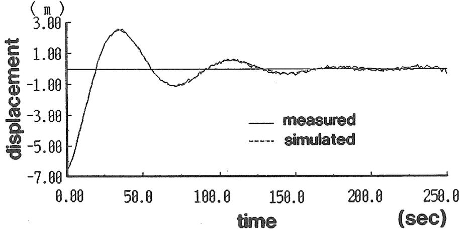
Fig. 4.8 Comparison between full-scale surge decaying time history and the simulation result obtained from the present identification taking into account the *Keulegan-Carpenter* number dependence of drag coefficient
