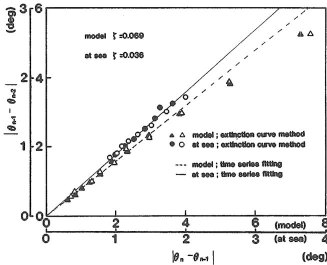
Fig. 4.9 Extinction curve of full-scale pitch decaying motion
