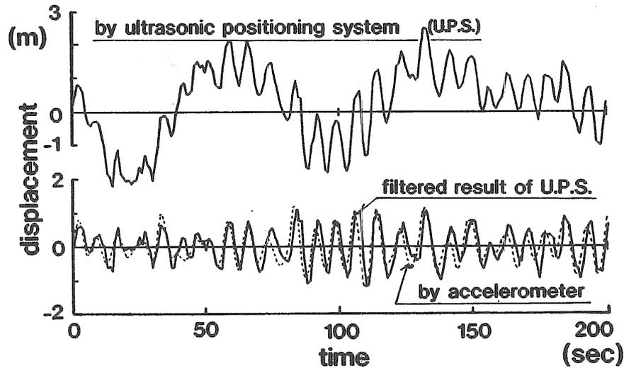
Fig. 2.8 Comparison of measured surge time histories between by accelerometer and by ultrasonic type position measuring system
