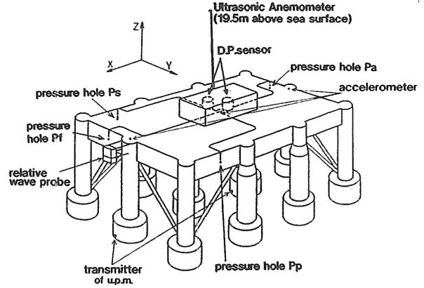
Fig. 2.4 Wind pressure measurement system
