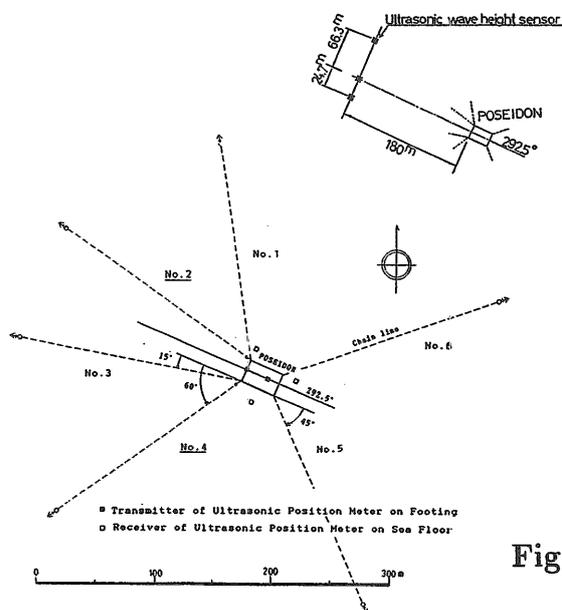
Fig. 2.3 Set-up of mooring system and wave measurement system
