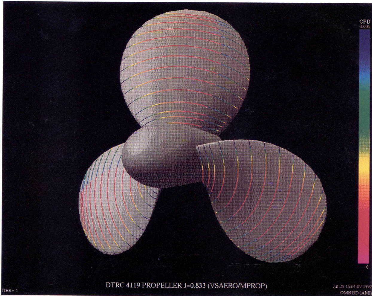
Fig. 4.7. Calculated Skin Friction Distribution Along Streamlines at J = 0.833 (a) VSAERO/MPROP
