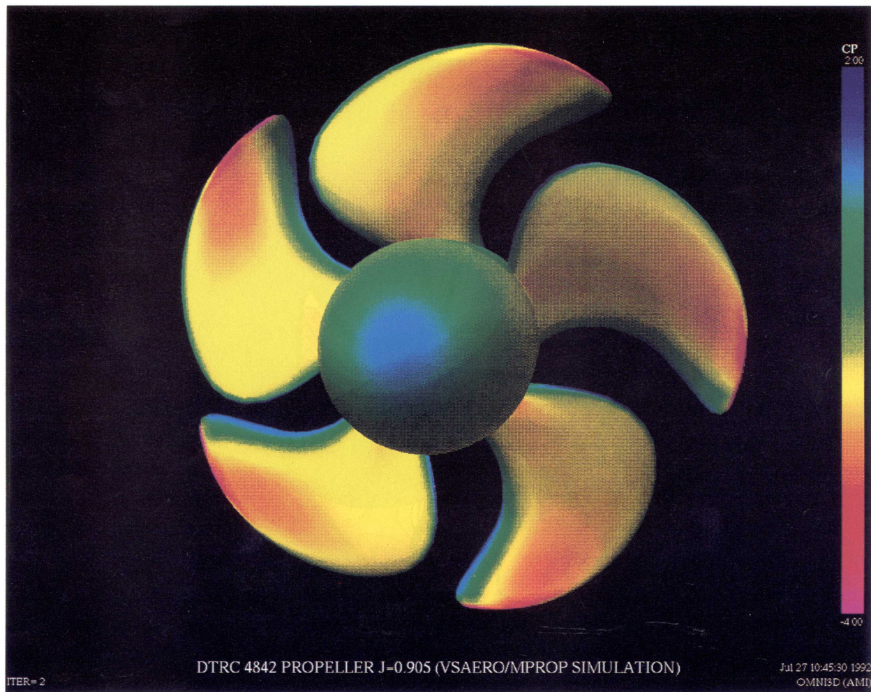
Fig. 4.9. Calculated Pressure Contours at J = 0.905 (a) VSAERO/MPROP
