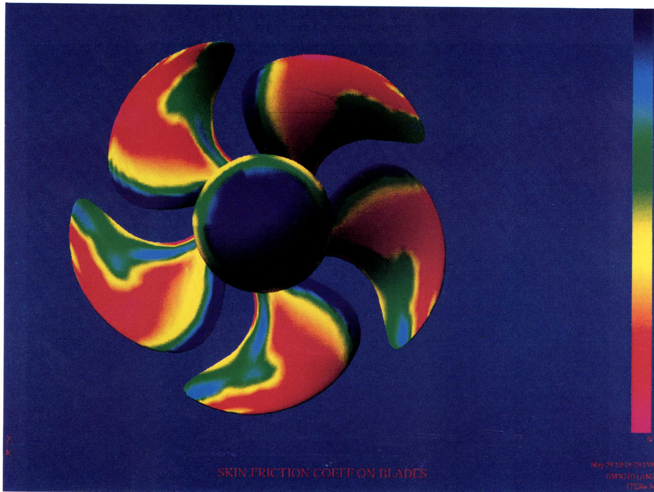
Fig. 4.13. Concluded. (c) As Surface Contours in USAERO
