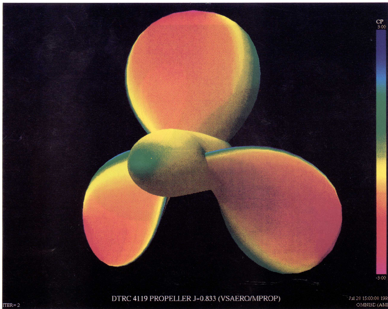
Fig. 4.2. Calculated Pressure Contours at J = .833 (a) VSAERO/MPROP
