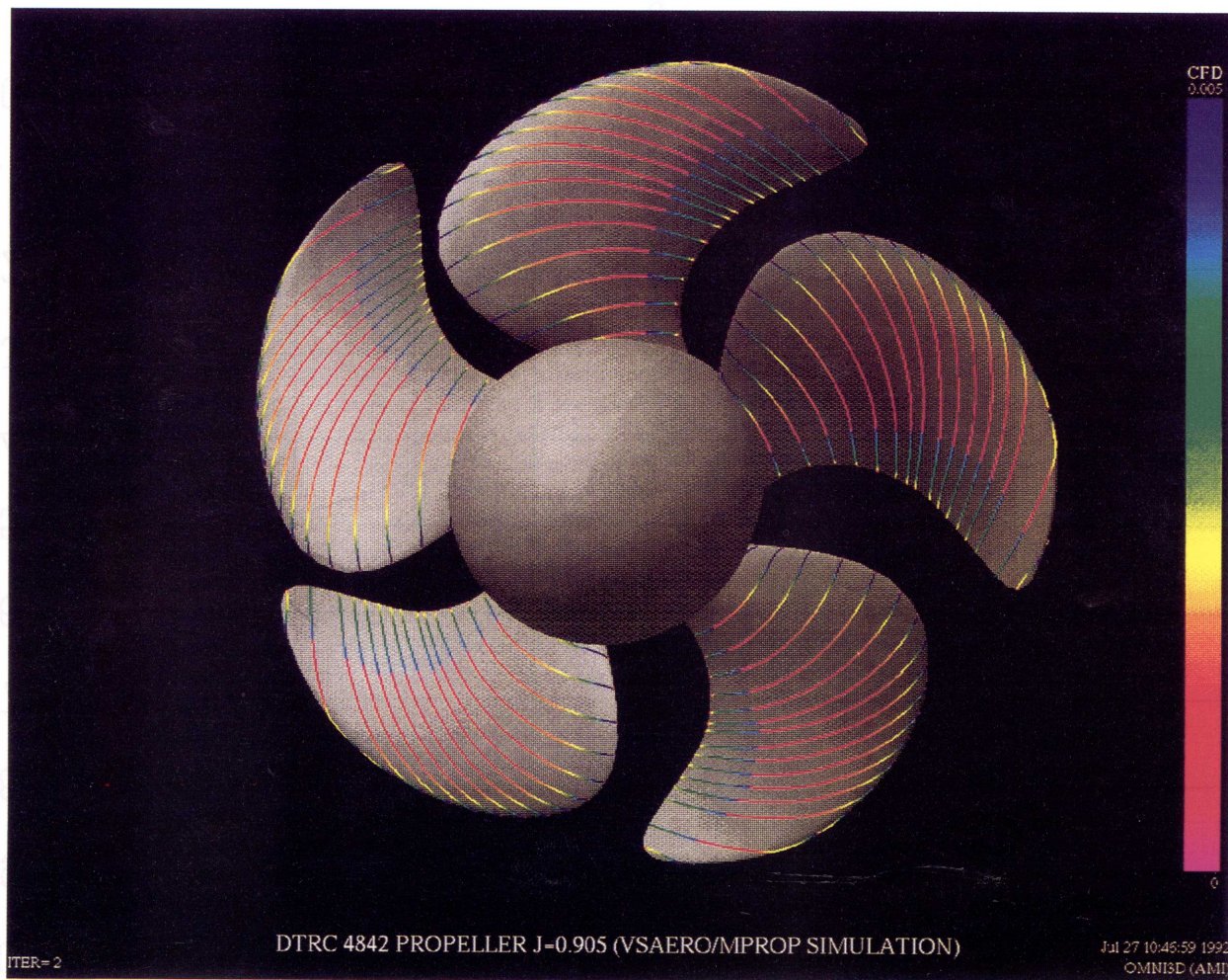
Fig. 4.13. Calculated Skin Friction Distribution at J = 0.905 (a) Along Streamlines in VSAERO/MPROP.
