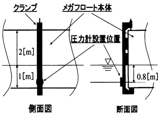
Fig. 19: A pressure gage fixed to Phase II Model
