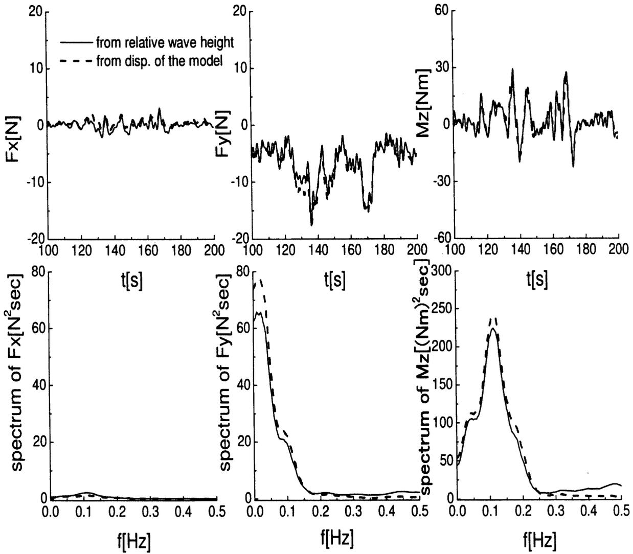
Fig. 9: Comparison of slowly varying drift forces estimated from relative wave height and disp. of the model
