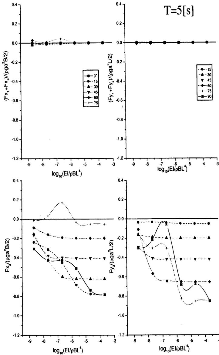
Fig. 2: Steady wave drift force due to (the 1st + the 2nd term) and the 3rd term of eq.(20)(T=5sec.)
