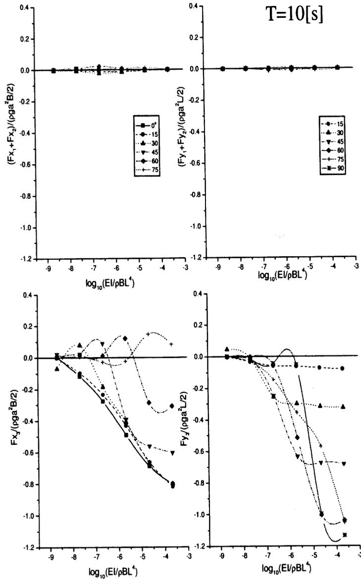
Fig. 3: Steady wave drift force due to (the 1st + the 2nd term) and the 3rd term of eq.(20)(T=10sec.)
