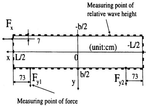
Fig. 5: Measuring points of relative wave height & force
