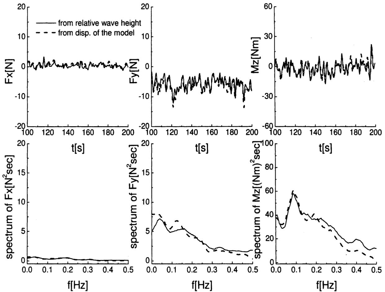
Fig. 10: Comparison of slowly varying drift forces estimated from relative wave height and disp. of the model  $S_{max} = 10, \theta = 60[\text{deg}]$
