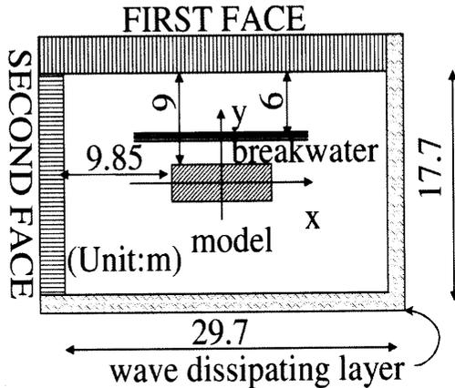
Fig. 8: Plane view of the model in the water tank
