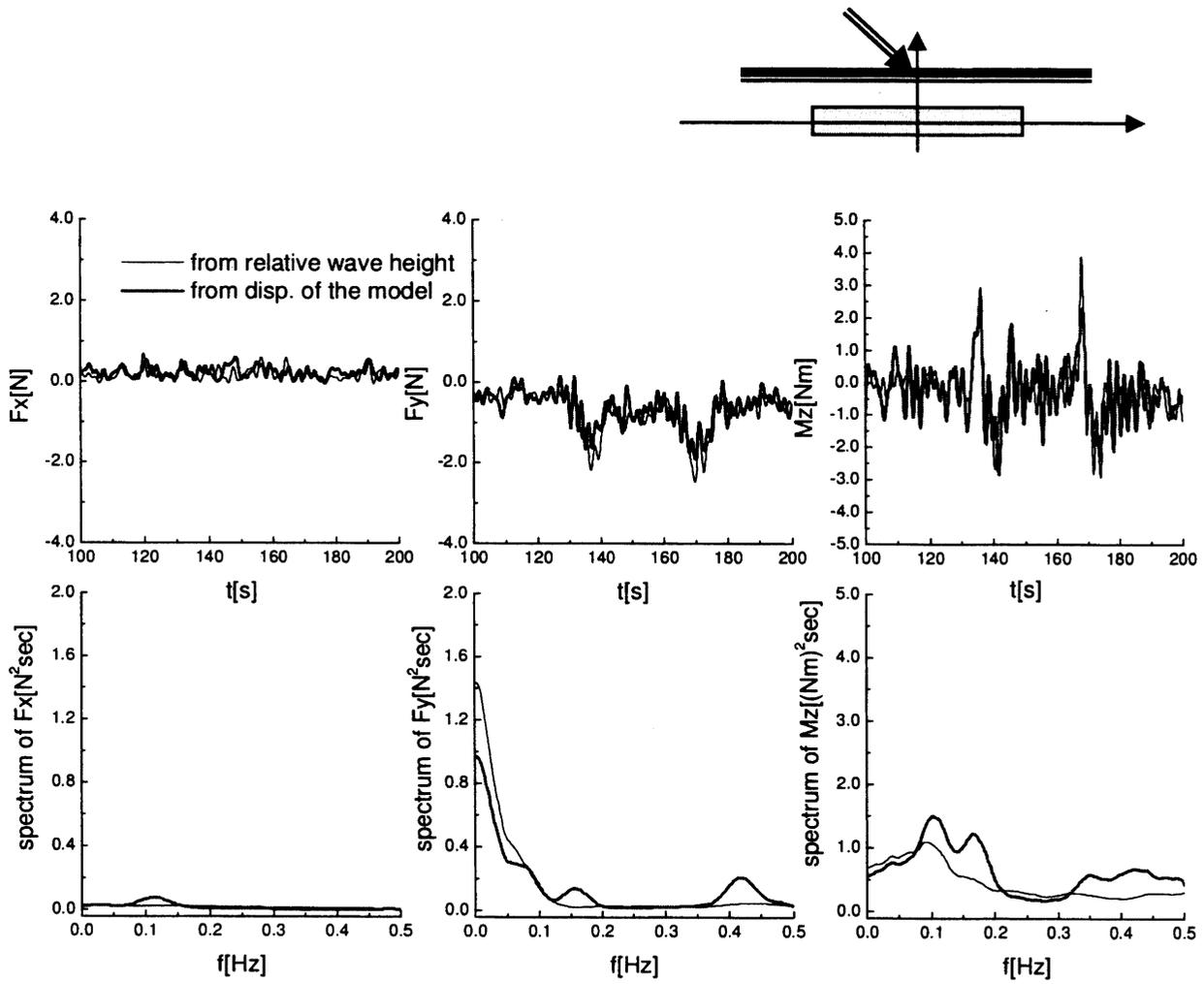
Fig. 14: Comparison of slowly varying drift forces estimated from relative wave height and disp. of the model (with break water)  $S_{max} = \infty, \theta = 120[\text{deg}]$
