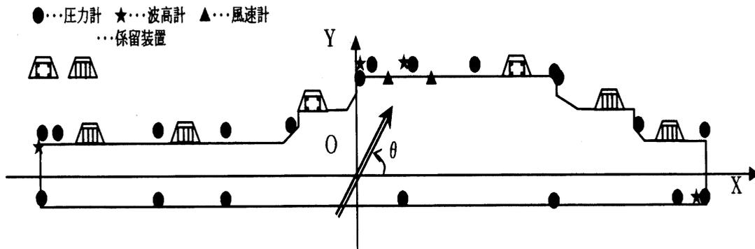
Fig. 17: Schematic view of Phase II Model, mooring system, and measurements
