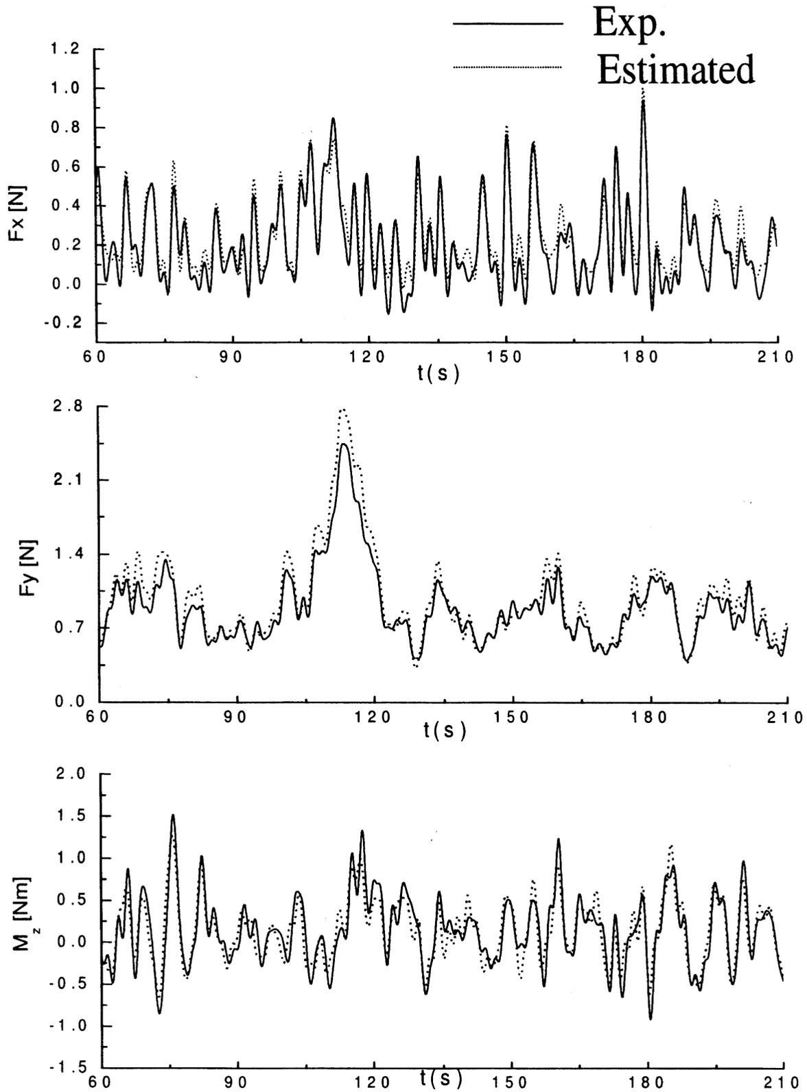
Fig. 6: Each component( $F_x, F_y, M_z$ ) of a slowly varying drift force in time domain (CASE1)
