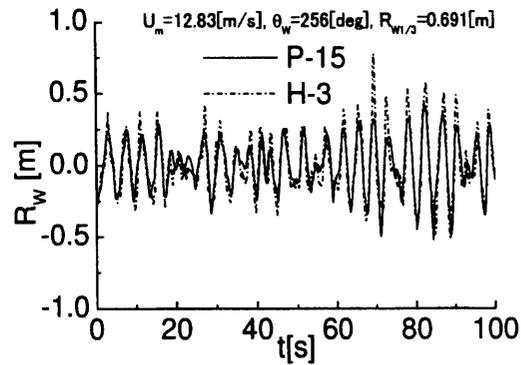
Fig. 20: Comparison of measured and estimated relative wave height
