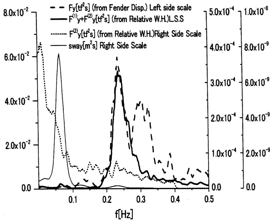
Fig. 21: Spectrum of sway displacement  $y$ , sway wave force  $F_y$  on
