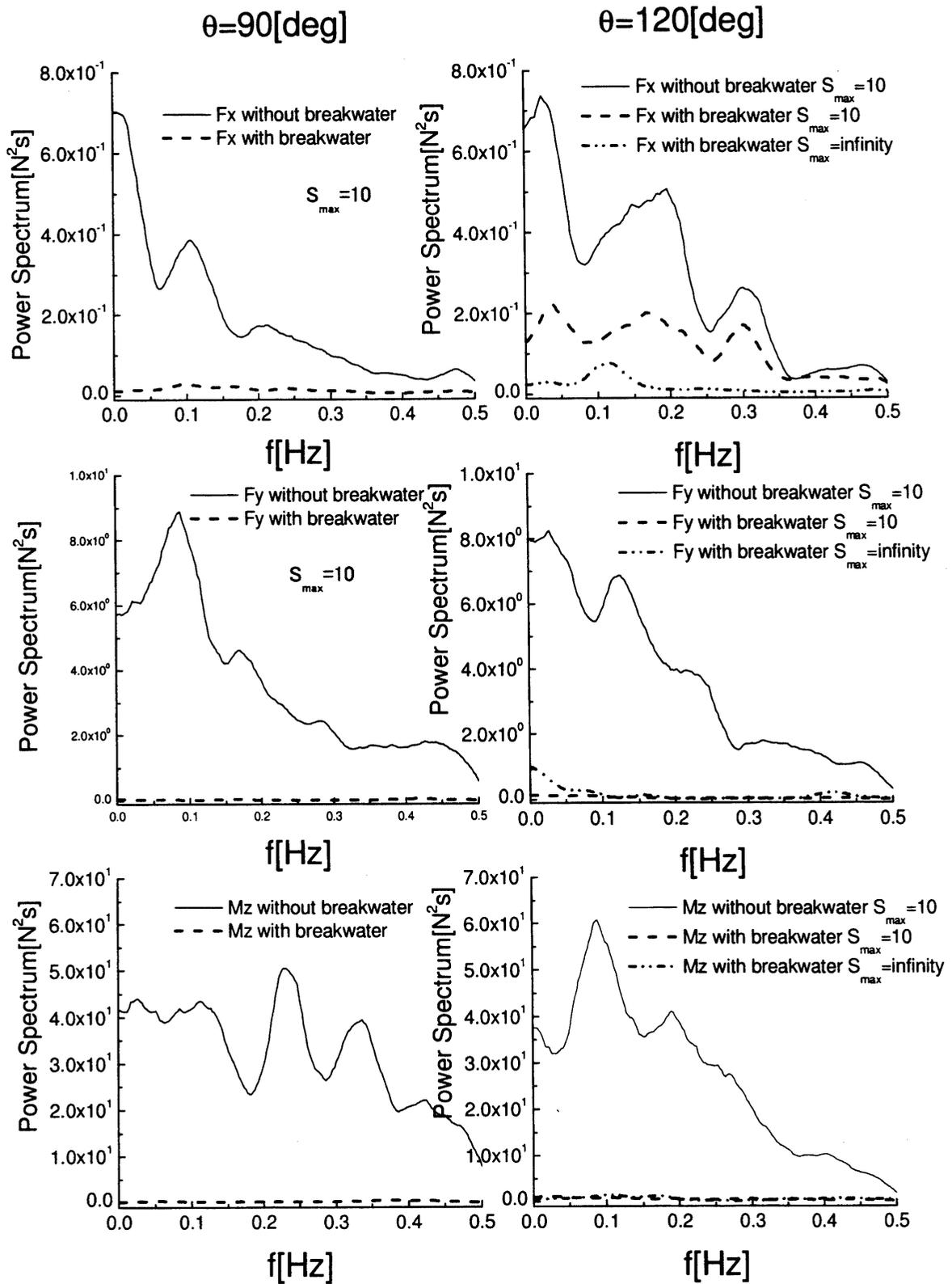
Fig. 13: Break water effect for slowly varying drift forces
