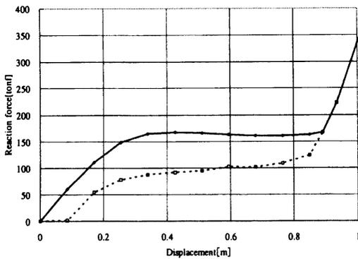
Fig. 18: Dimensionless reaction force of fender
