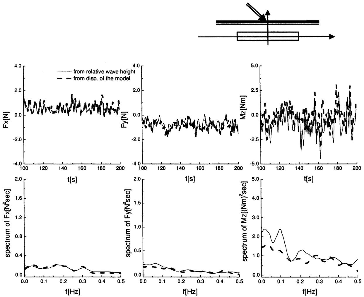
Fig. 15: Comparison of slowly varying drift forces estimated from relative wave height and disp. of the model (with break water)  $S_{max} = 10, \theta = 120$  [deg]
