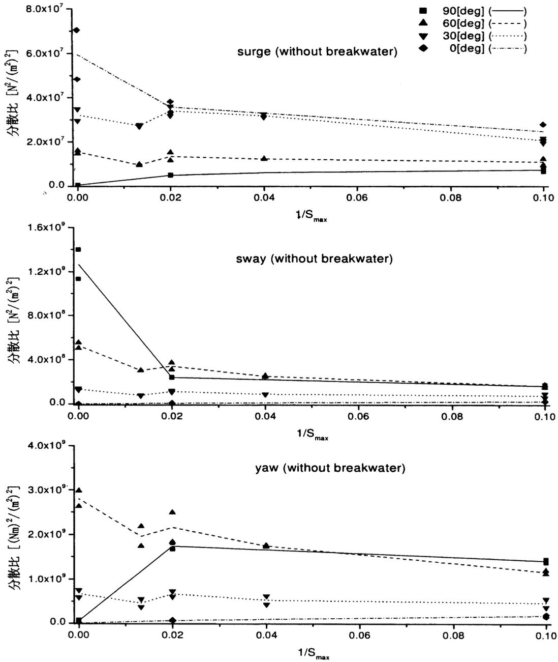
Fig. 12: Change of variances of slow drift forces with respect to directional spreading parameter  $S_{max}$  of waves
