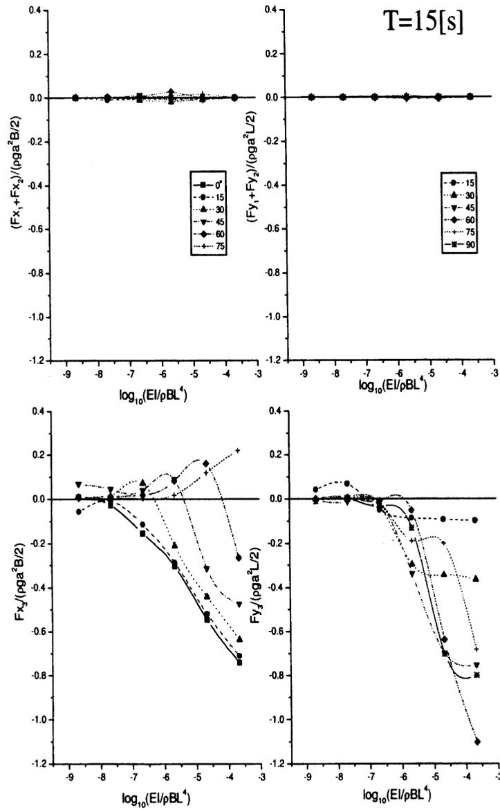
Fig. 4: Steady wave drift force due to (the 1st + the 2nd term) and the 3rd term of eq.(20)( $T=15$ sec.)
