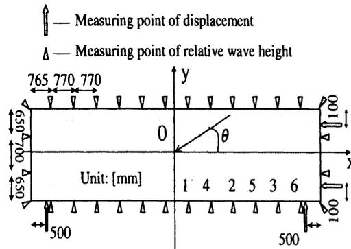
Fig. 7: Measuring points of relative wave height & force
