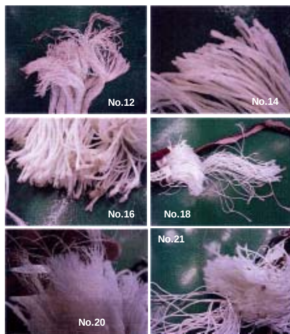
Photo. 2.2.1-12 Appearance of breakage parts of towline at first tow operation
