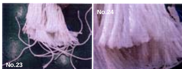
Photo. 2.2.1-17 Appearance of breakage parts of towline cut by knife
