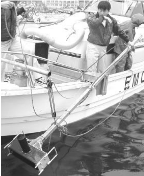
Photo2.1.4-1 Example of multibeam echosounder.
