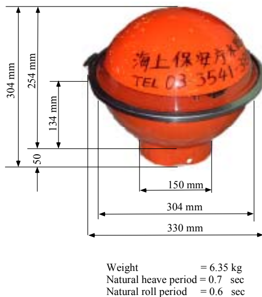
Fig. 2.1.2-6 Spherical buoy used for the measurement.
