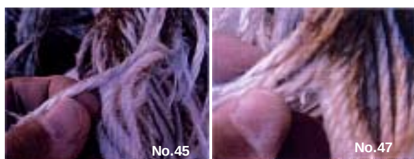
Photo. 2.2.1-18 Appearance of breakage parts of towline at first tow operation
