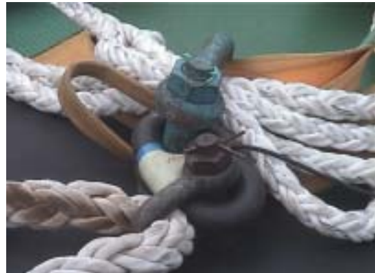
Photo 2.2.2-1 Tension meter installed at bow.
