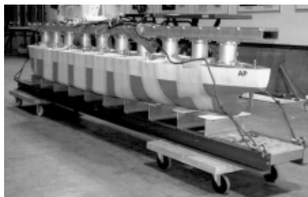
Photo2.1.3-1 Experimental model that divided VLCC.
