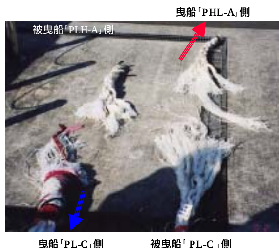
Photo. 2.2.1-11 Appearance of breakage parts of towline
