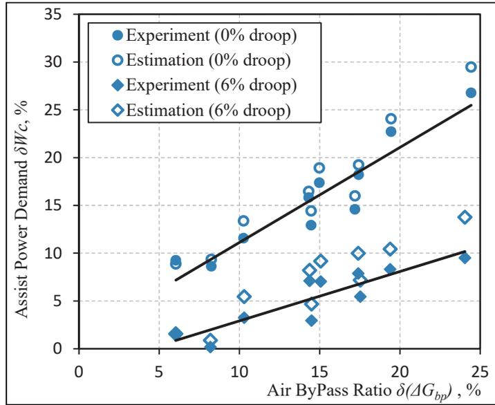
Fig. 8 Assist power demand for astatic and droop control
