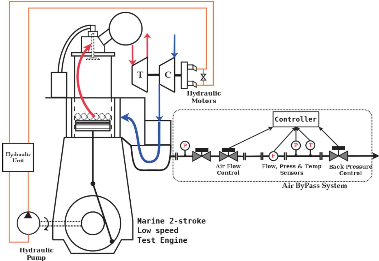
Fig. 7 Test engine equipped with the air bypass and TCH assist systems
