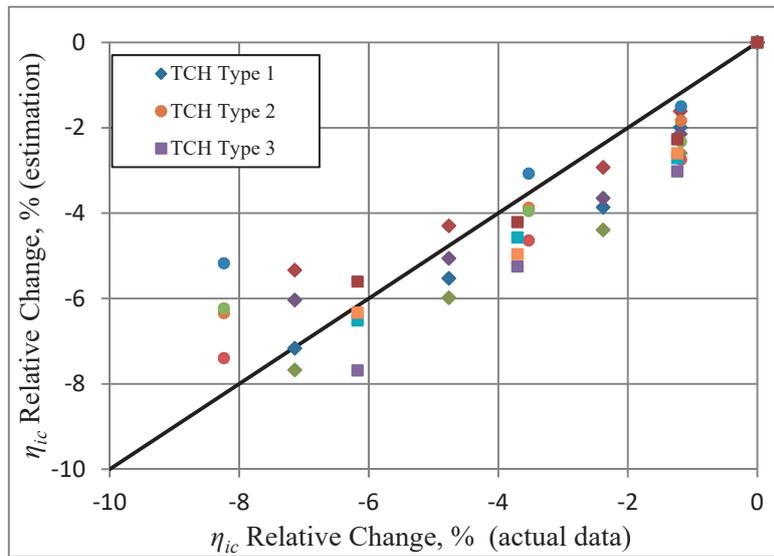
Fig. 5 Compressor efficiency relative deviation; estimated and experimental
