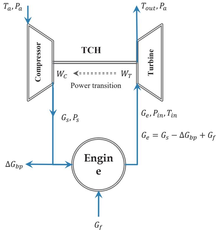
Fig. 2 Schematic of TCH-Engine interaction
