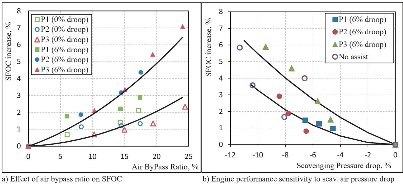
a) Effect of air bypass ratio on SFOC
