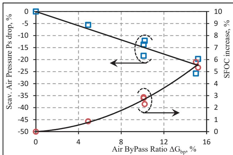
Fig. 4 Effect of scavenging air bypass on the engine performance
