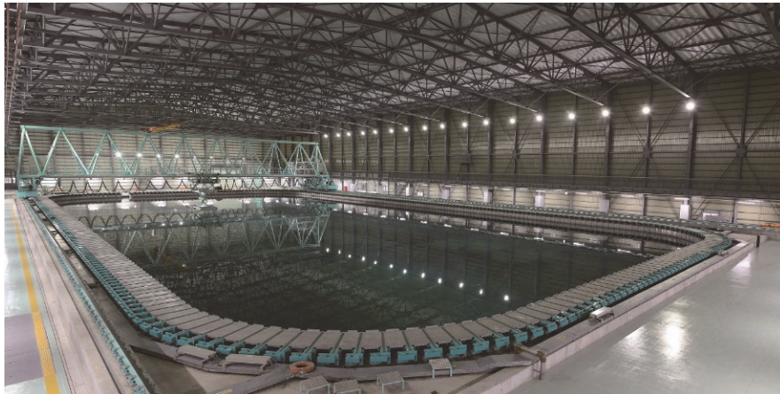
Fig. 2 Actual Sea Model Basin of the NMRI, measuring 80.0 m (length) × 40.0 m (width) × 4.50 m (depth).
