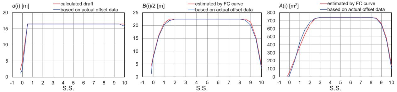
Fig. 5 Validation for sectional parameters of JBC
