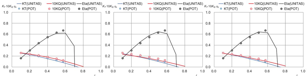
Fig. 9 Validation for POC of 499GT cargo ship
