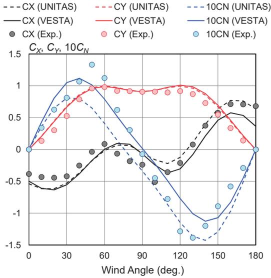
Fig. 17 Validation for vehicle carrier ( $L_{OA} = 199$  m)
