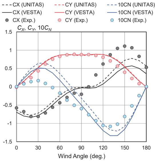
Fig. 15 Validation for container ship ( $L_{OA} = 312$  m)
