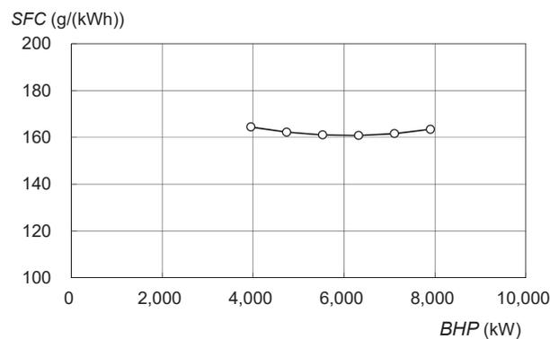
Fig. 23 Specific fuel oil consumption (SFC) of engine
