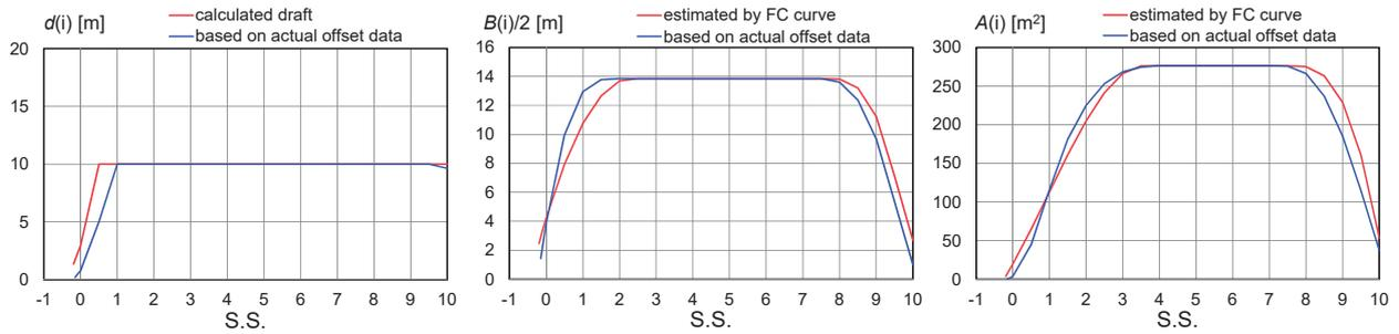
Fig. 4 Validation for sectional parameters of 33CT
