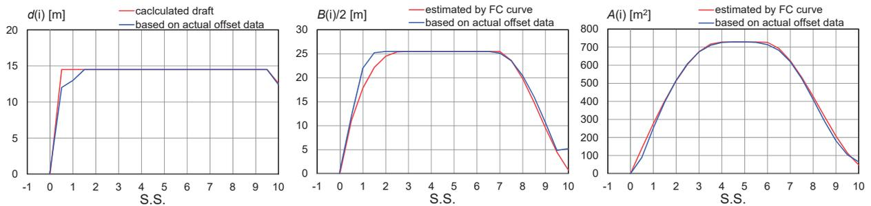
Fig. 6 Validation for sectional parameters of DTC
