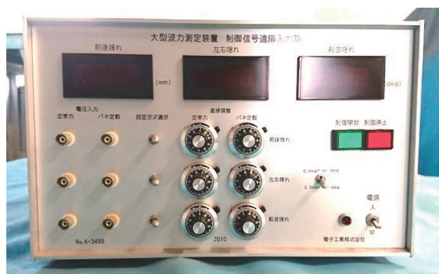
Fig. 2 Control panel for restoring forces and steady forces.
