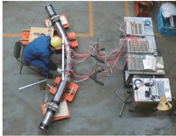
Fig. 5 Bending test of the multilayered pipe model
