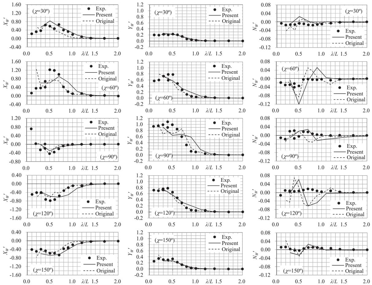
Fig. 14 Steady wave loads of a sample tanker depending on wavelength to ship length ratio estimated by present program (Present), 3D panel method (Original), and experimental data (Exp.)
