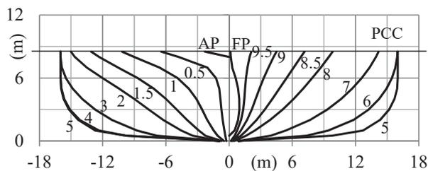
Fig. 3 Body plan of type ship, PCC
