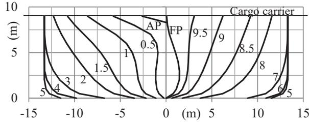
Fig. 4 Body plan of type ship, cargo carrier.
