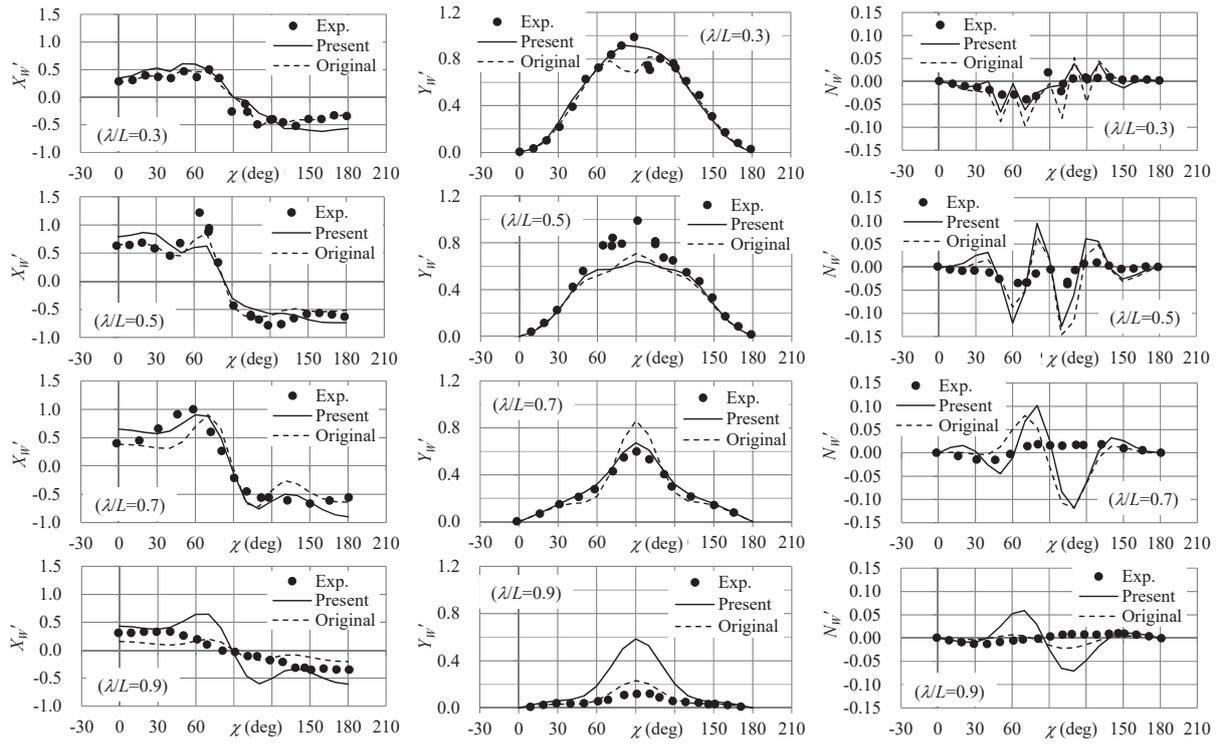
Fig. 15 Steady wave loads of a sample tanker depending on wave encounter angle estimated by present program (Present), 3D panel method (Original), and experimental data (Exp.)
