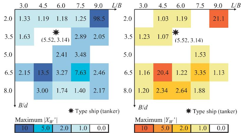
Fig. 8 Distribution of maximum  $|X_W'|$  and  $|Y_W'|$  larger than 1.0 (tanker)
