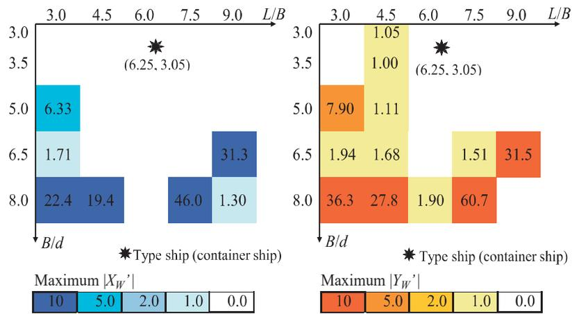
Fig. 9 Distribution of maximum  $|X_W'|$  and  $|Y_W'|$  larger than 1.0 (container ship).
