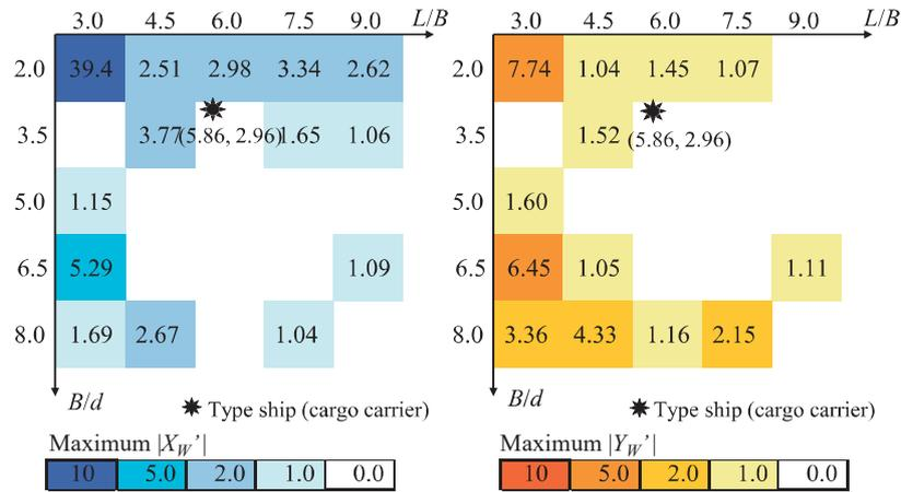
Fig. 11 Distribution of maximum  $|X_w'|$  and  $|Y_w'|$  larger than 1.0 (cargo carrier).
