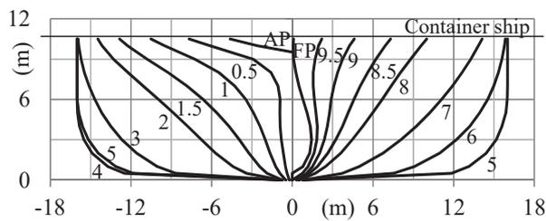
Fig. 2 Body plan of type ship, container ship
