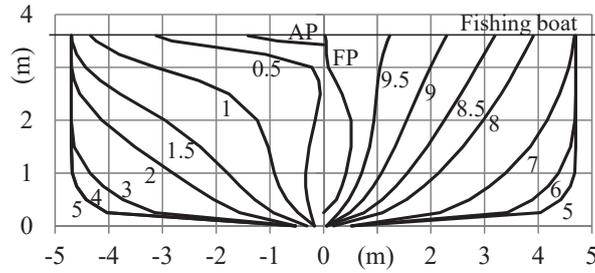
Fig. 5 Body plan of type ship, fishing boat.
