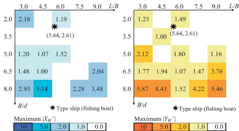
Fig. 12 Distribution of maximum  $|X_w'|$  and  $|Y_w'|$  larger than 1.0 (fishing boat).
