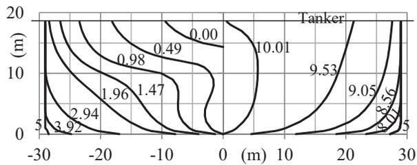
Fig. 1 Body plan of type ship, tanker.
