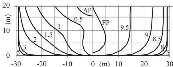
Fig. 13 Body plan of sample ship, tanker.
