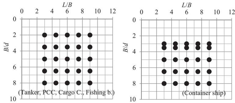
Fig. 6 Combination of  $L/B$  and  $B/d$  of modified ship forms for calculation (Left; tanker, PCC, cargo carrier, and fishing boat; Right; container ship).
