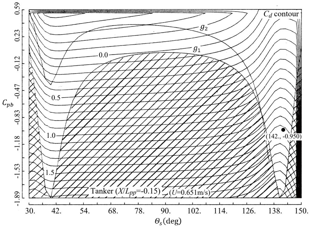
Fig. 4.3.13 Tanker's  $C_d(\theta_s, C_{pb})$  at  $X/L_{pp} = -0.15$ .
