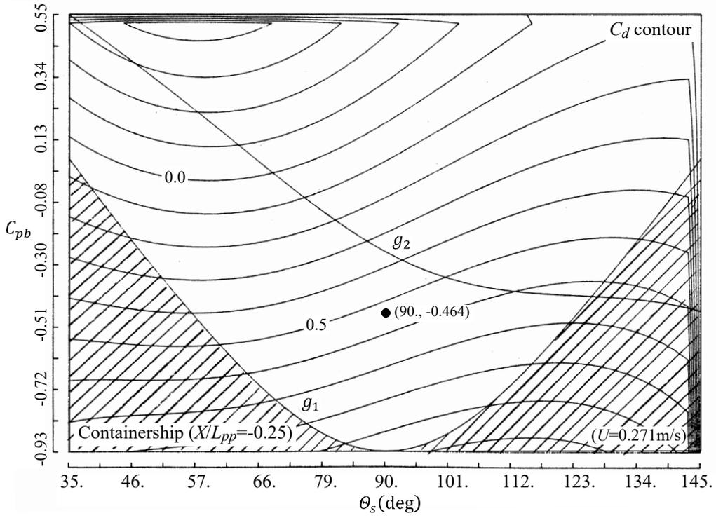
Fig. 4.3.8 Containership's  $C_d(\theta_s, C_{pb})$  at  $X/L_{pp} = -0.25$ .
