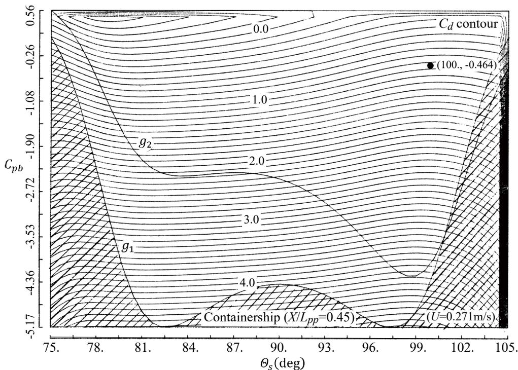
Fig. 4.3.1 Containership’s  $C_d(\theta_s, C_{pb})$  at  $X/L_{pp}=0.45$ .
