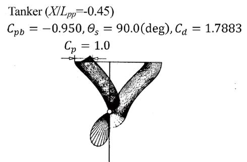
Fig. 4.2.15 Tanker's sectional flow and  $C_p$  at  $X/L_{pp}=-0.35$ .
