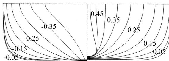
Fig. 4.1.2 Containership body plan approximated by Lewis form.
