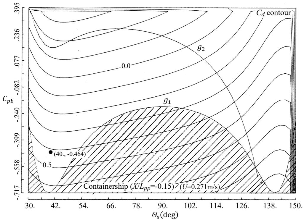
Fig. 4.3.7 Containership's  $C_d(\theta_s, C_{pb})$  at  $X/L_{pp} = -0.15$ .
