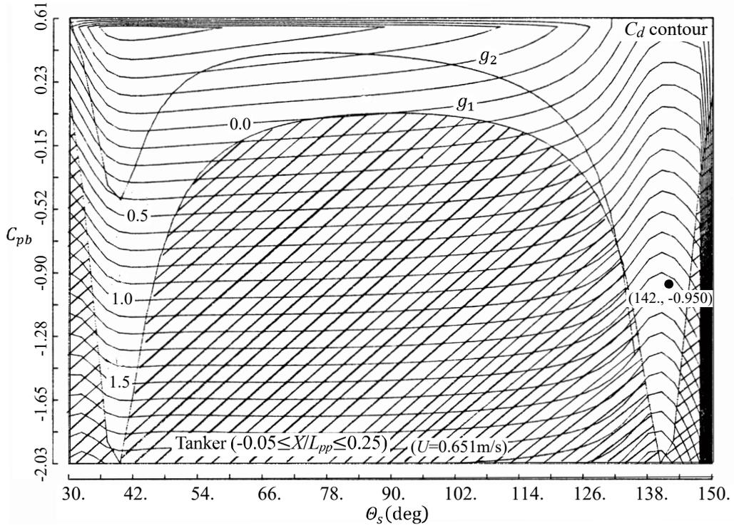
Fig. 4.3.12 Tanker's  $C_d(\theta_s, C_{pb})$  at  $-0.05 \leq X/L_{pp} \leq 0.25$ .
