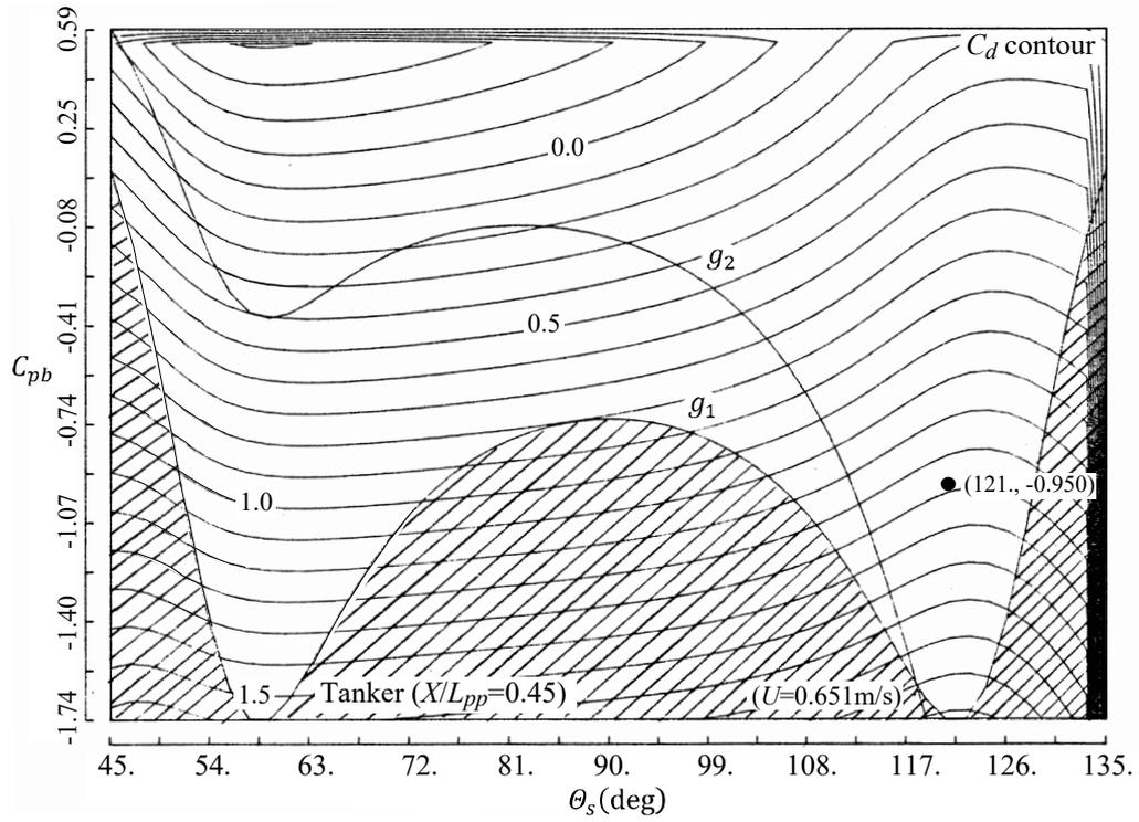
Fig. 4.3.10 Tanker's  $C_d(\theta_s, C_{pb})$  at  $X/L_{pp}=0.45$ .
