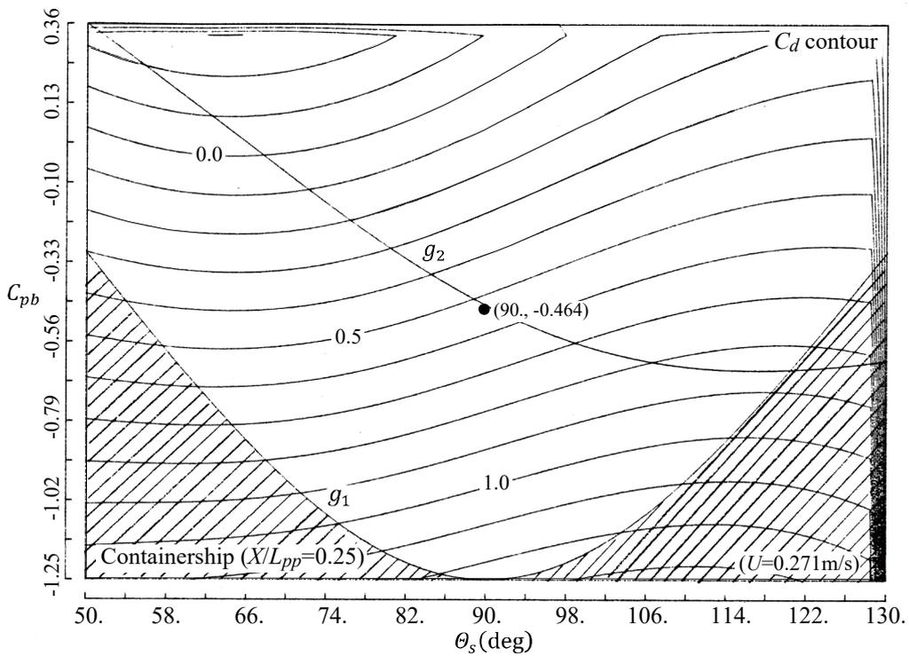
Fig. 4.3.3 Containership's  $C_d(\theta_s, C_{pb})$  at  $X/L_{pp}=0.25$ .
