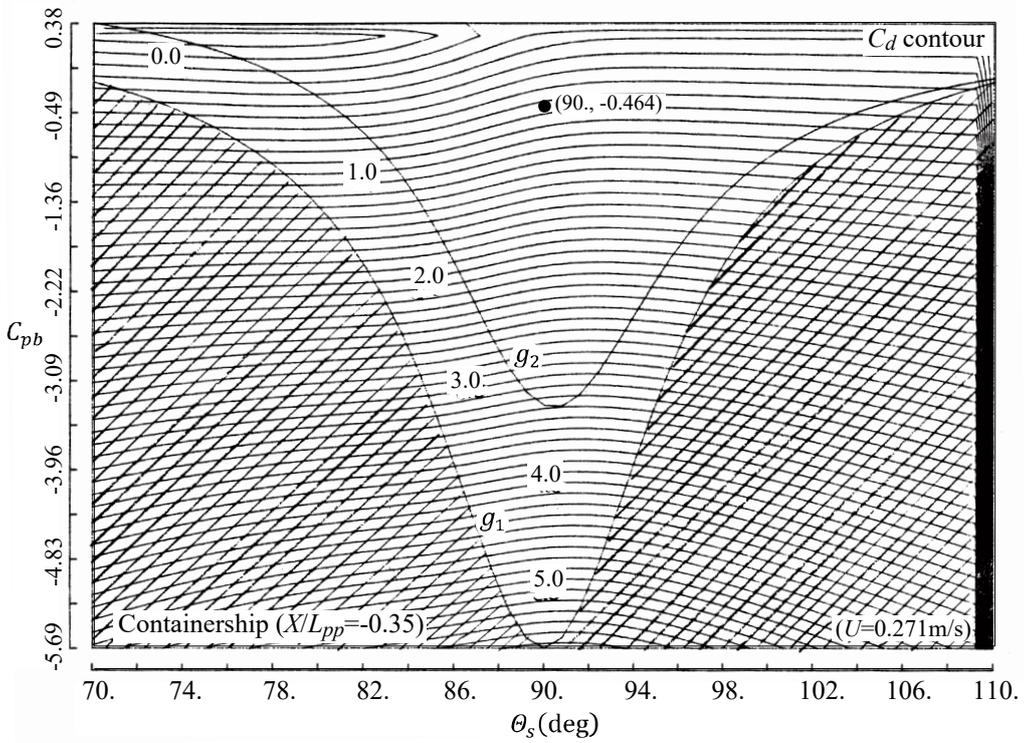
Fig. 4.3.9 Containership's  $C_d(\theta_s, C_{pb})$  at  $X/L_{pp} = -0.35$ .
