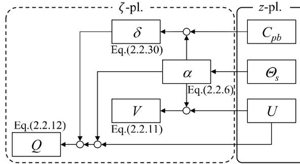
Fig. 2.2.2 Relation between variables in the z-pl. and those in the ζ-pl. for the wake source model.
