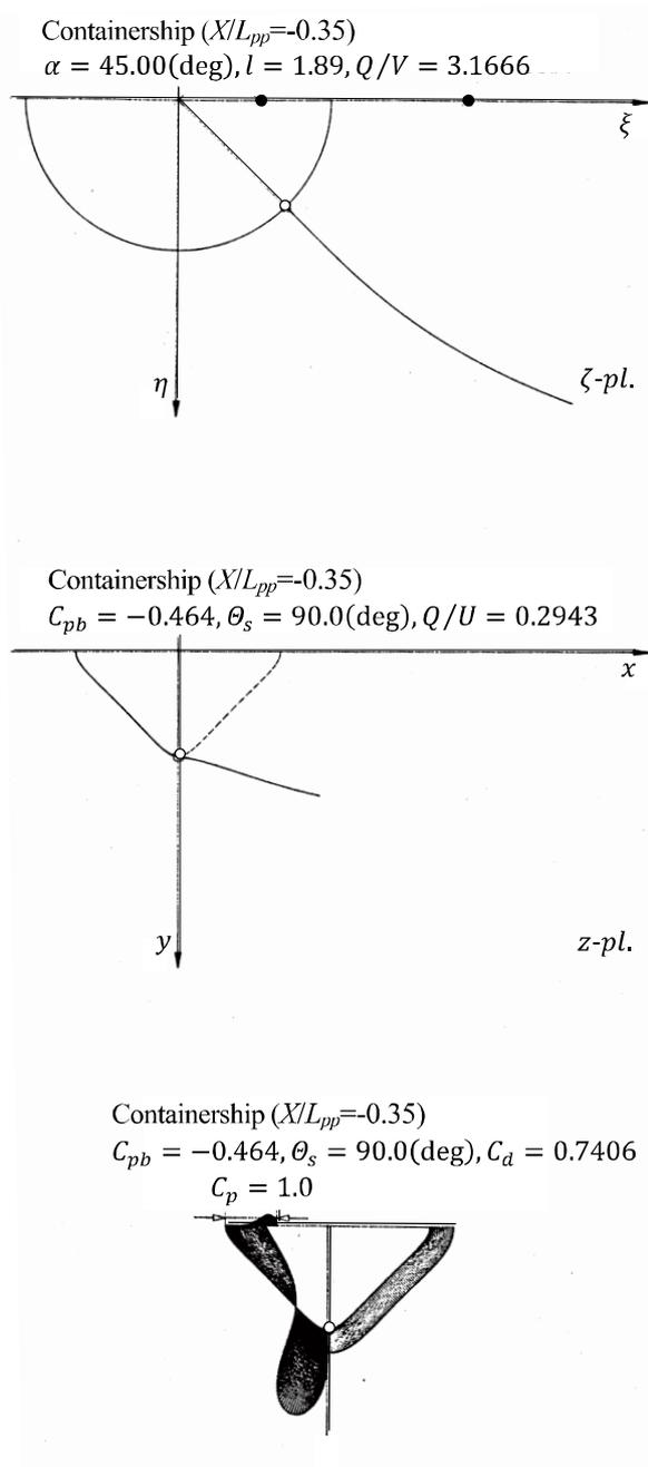
Fig. 4.2.9 Containership's sectional flow and  $C_p$  at  $X/L_{pp}=-0.35$ .
