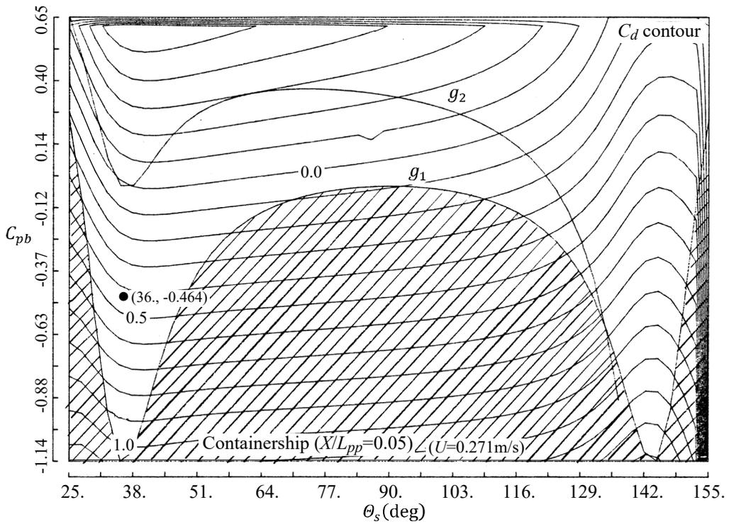
Fig. 4.3.5 Containership's  $C_d(\theta_s, C_{pb})$  at  $X/L_{pp} = 0.05$ .
