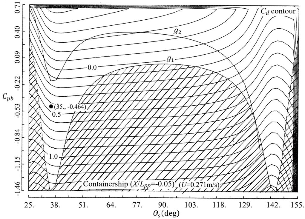
Fig. 4.3.6 Containership's  $C_d(\theta_s, C_{pb})$  at  $X/L_{pp} = -0.05$ .
