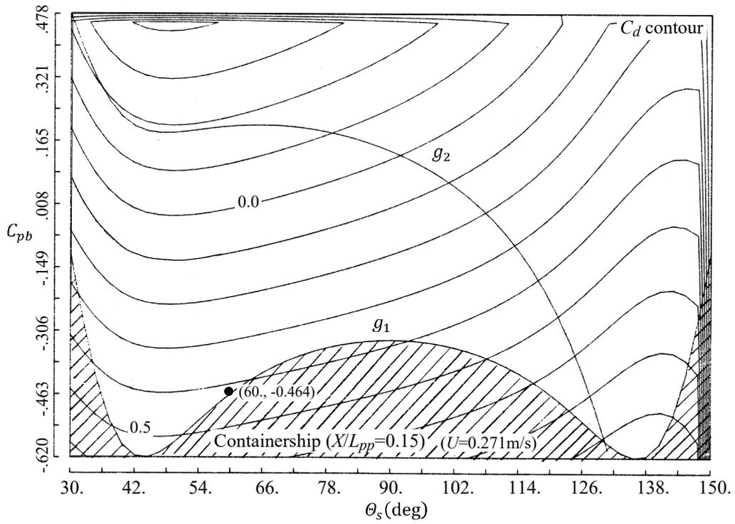
Fig. 4.3.4 Containership's  $C_d(\theta_s, C_{pb})$  at  $X/L_{pp} = 0.15$ .
