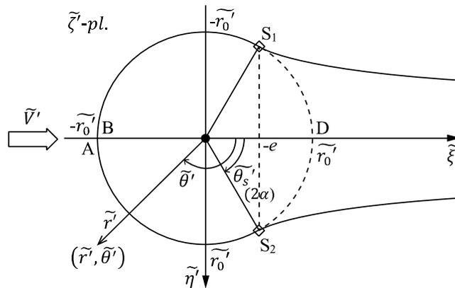
Fig. 2.1.2 Transformed separated flow around a circular cylinder with radius  $\widetilde{r}_0'$ ,  $\widetilde{\zeta}'$ -pl.
