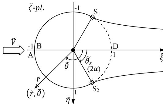
Fig. 2.1.3 Transformed separated flow around a circular cylinder with radius 1,  $\tilde{\zeta}$ -pl.
