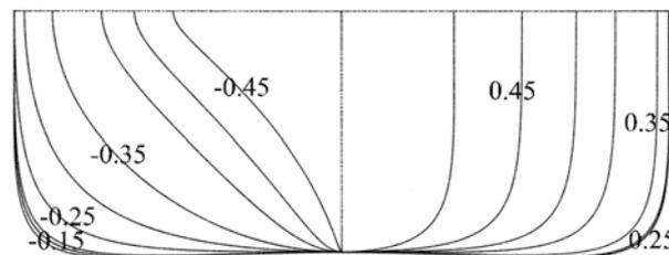
Fig. 4.1.3 Tanker body plan approximated by Lewis form.
