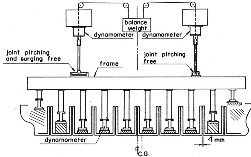
Fig. 4.1.1 Arrangement of the segmented model. Reprinted from Matsumoto and Suemitsu<sup>11)</sup> with permission from The Japan Society of Naval Architects and Ocean Engineers.
