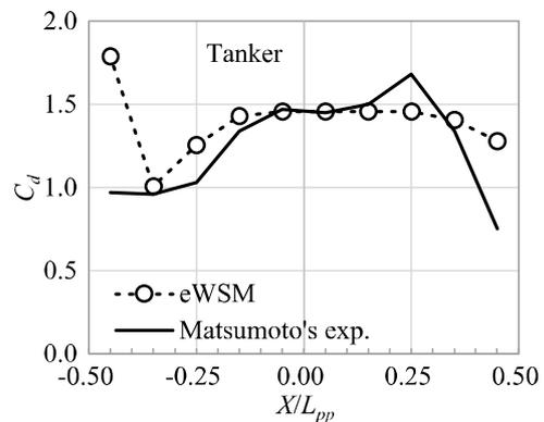
Fig. 4.4.2  $C_d$  distribution of tanker.
