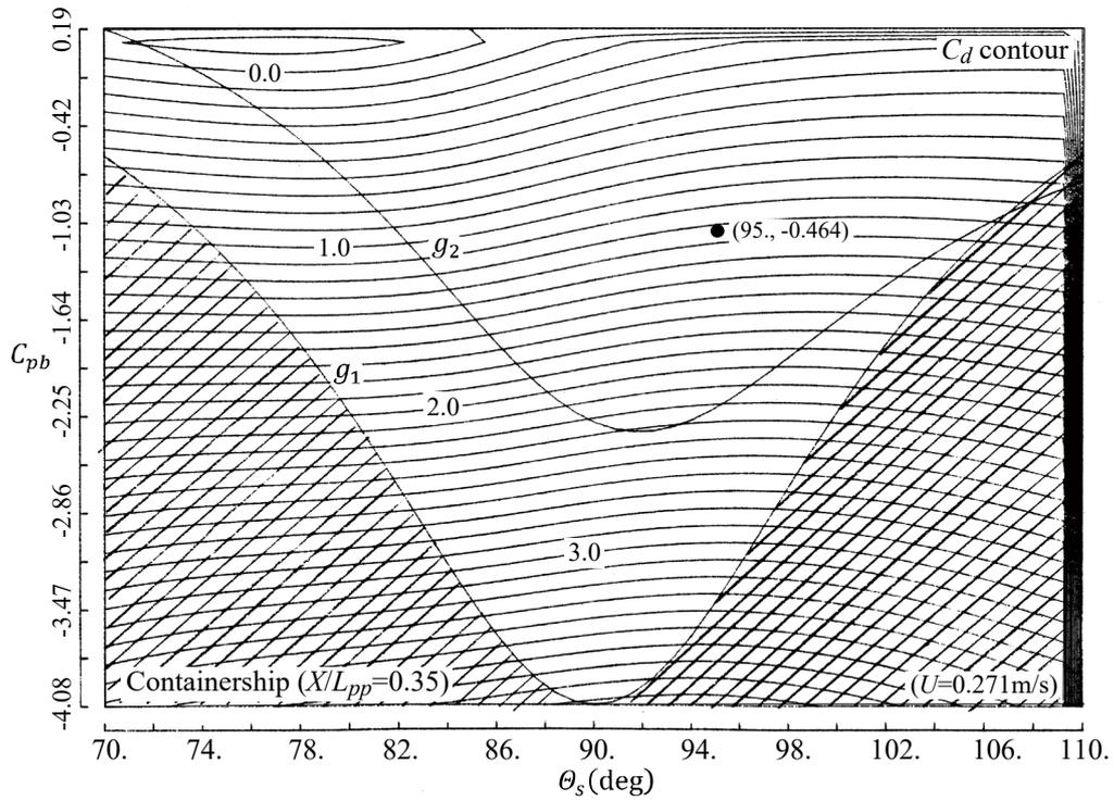
Fig. 4.3.2 Containership's  $C_d(\theta_s, C_{pb})$  at  $X/L_{pp}=0.35$ .
