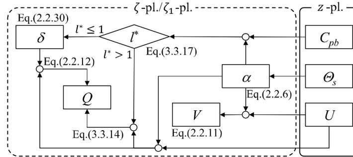
Fig. 3.3.3 Relation between variables in the  $z$ -pl., and those in the  $\zeta$ - or  $\zeta_1$ -pl. for the enhanced wake source model.
