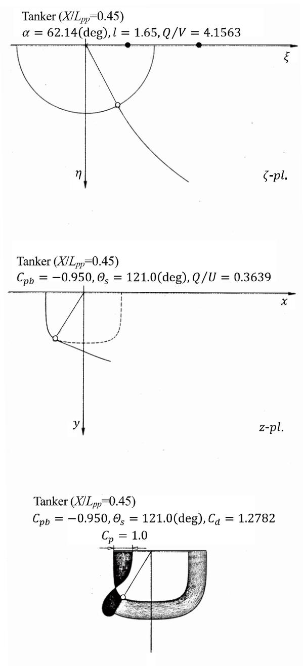
Fig. 4.2.10 Tanker's sectional flow and  $C_p$  at  $X/L_{pp}=0.45$ .
