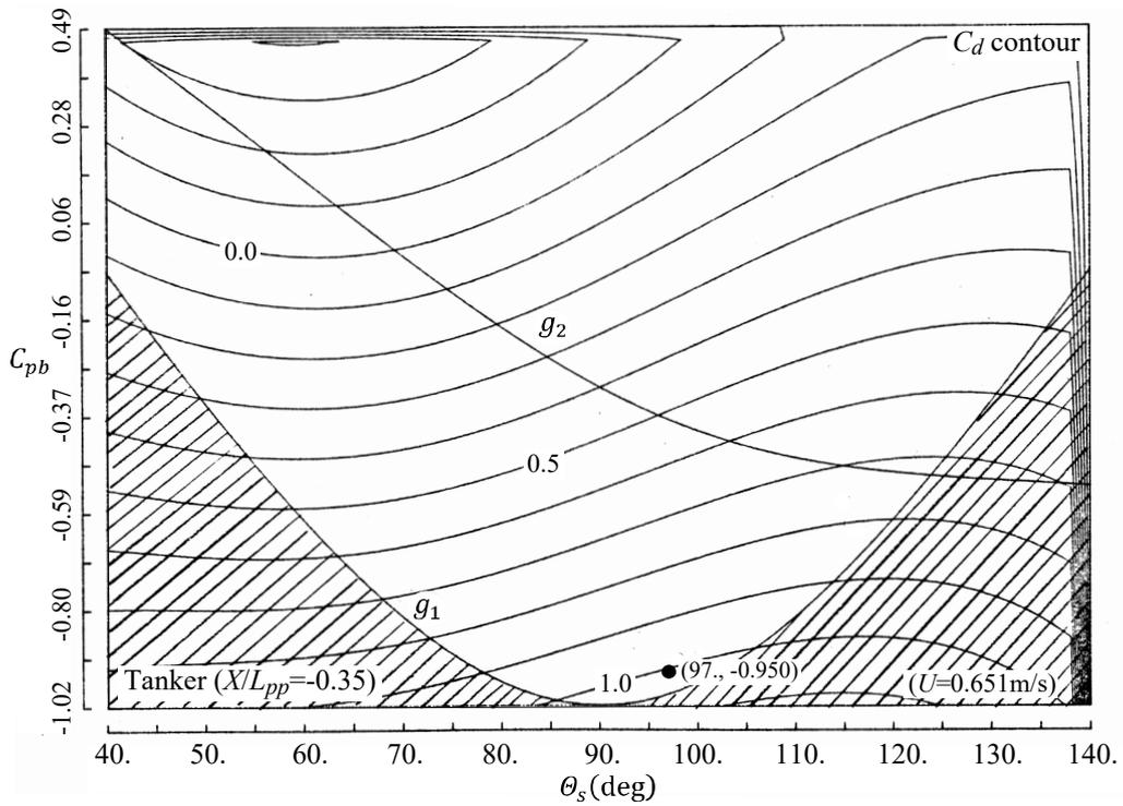
Fig. 4.3.15 Tanker's  $C_d(\theta_s, C_{pb})$  at  $X/L_{pp} = -0.35$ .
