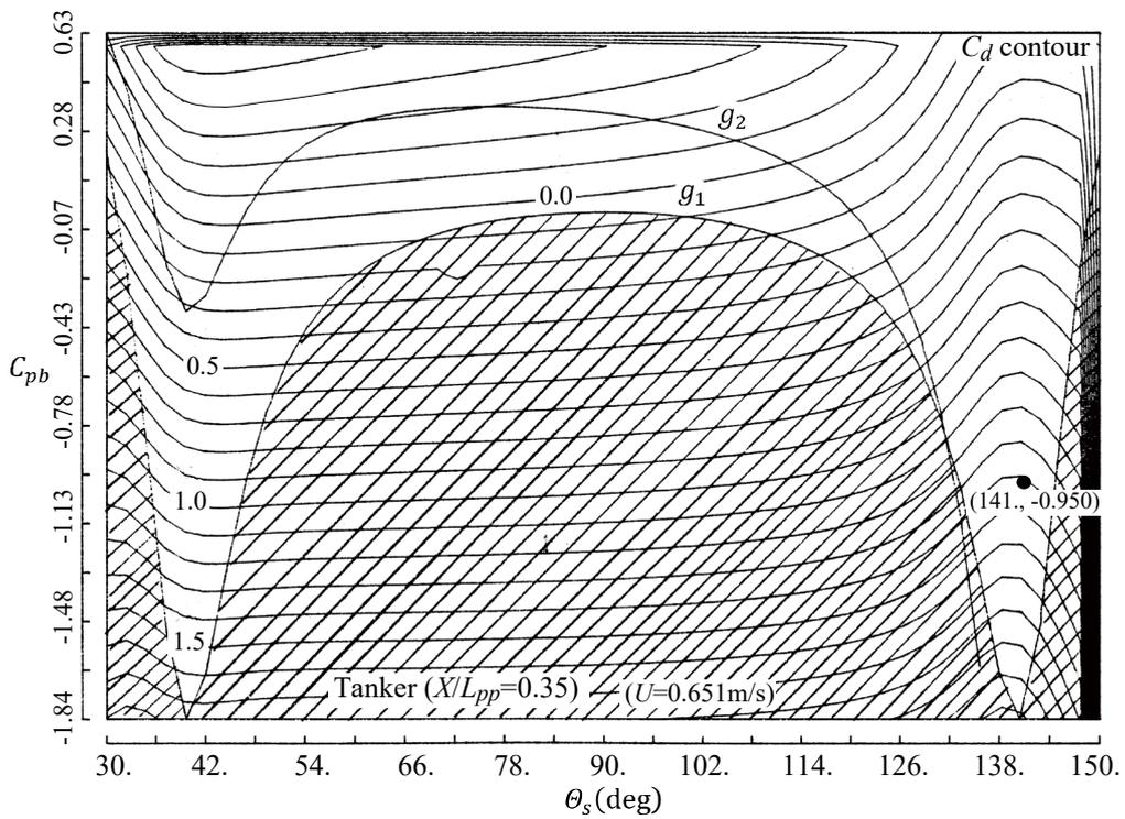
Fig. 4.3.11 Tanker's  $C_d(\theta_s, C_{pb})$  at  $X/L_{pp}=0.35$ .
