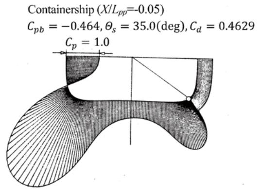
Fig. 4.2.5 Containership's sectional flow and  $C_p$  at  $X/L_{pp}=0.05$ .
