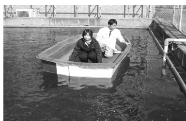
Float test of BFRP boat
