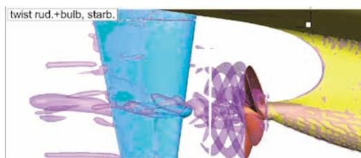
Fig. DTC vortical structure at stern,  $Fn=0.209$
