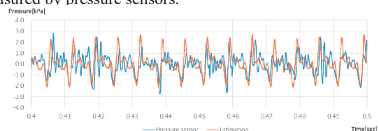
Figure Time series comparison of pressure fluctuation of pressure sensor and estimation.
