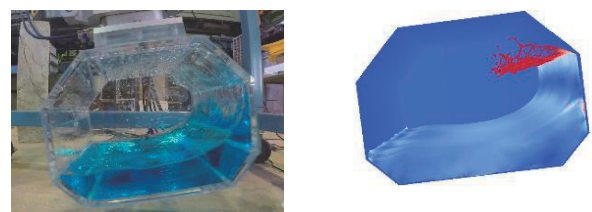
Fig.1 Comparison of free surface of roll sloshing between experiment and SPH
