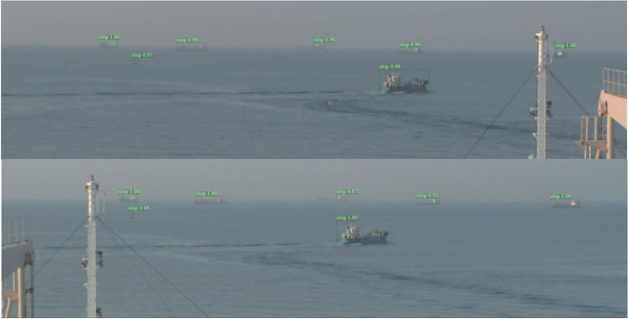
Fig. 4 Example Images of Detected Ships and Navigation Buoys. (Upper: Left Cam, Lower: Right Cam)
