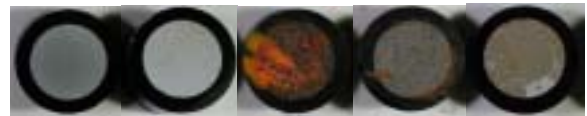
Fig. 1 Photographs of the coatings after an artificial-sea-water immersing corrosion test. From the left to Mullite, Al_2O_3 , TiO_2 , ZrO_2 and ZrSiO_4 .
