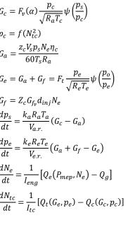
Fig.2 Engine model
