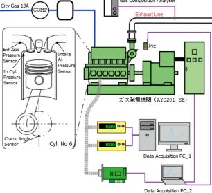
Fig.1 Engine data acquisition system
