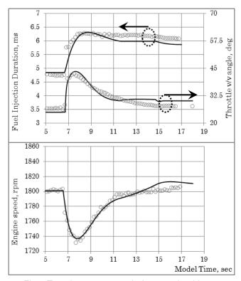
Fig.3 Transient response during step load input.
