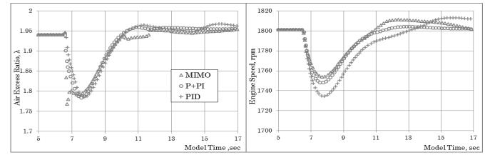
Fig.4 Effect of different control strategies on the gas engine transient dynamic
