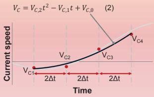
2. ship's speeds over ground at one power setting are expressed as follows using formula (2):
