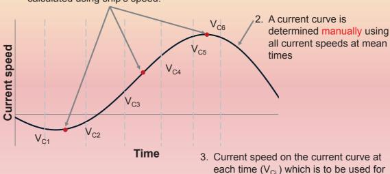
The process in which current curve is fitted manually involves arbitrariness and ambiguity.
