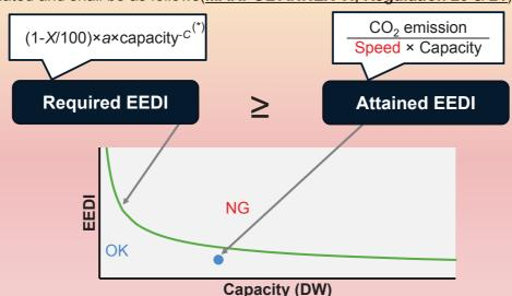
Speed in the attained EEDI is ship's speed in the ideal condition assuming the weather is calm with no wind, no current and no waves and the site is at the deep water of standard temperature/density.
