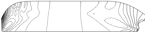
Fig.9: Cp contour maps on hull for original Grid4 ( \Delta Cp = 0.05 ).
